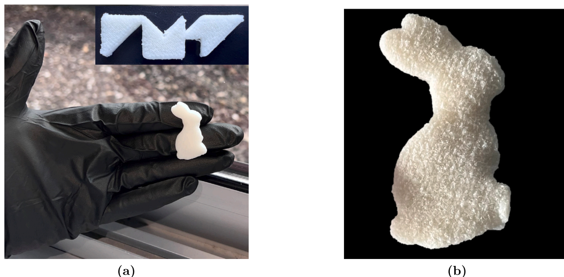
Fig. 8. Bunny and IMT logo printed using 5CP10SSG formulation (a), and bunny left at room temperature overnight (b).
