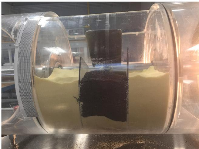
Fig. 5. Tracer initial position in the C-lab mixer.
