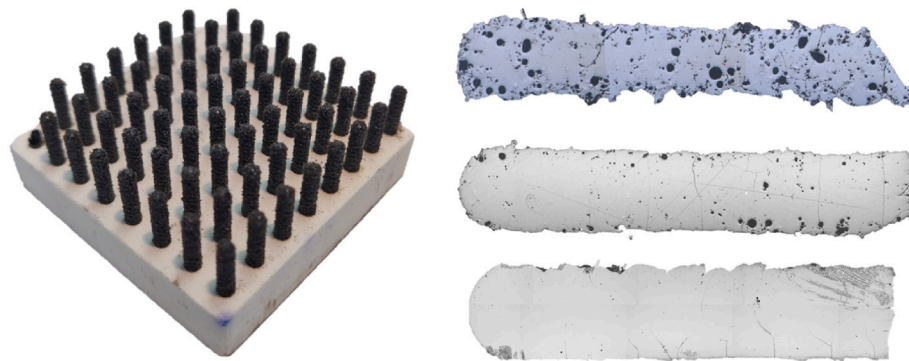
Fig. 13. (left) typical batch of 10 mm high and 3 mm diameter cylinders fabricated by SLM on their vitreous silica substrate and (right) cross sections in optical microscopy of such cylinders made with respectively 100 % native crystalline BPY powder (top, C/S configuration), with a mix of 50 wt% native crystalline BPY/50 wt% amorphous BPY (middle, CA/S configuration), 100 % amorphous BPY powder (bottom, A/S configuration).
