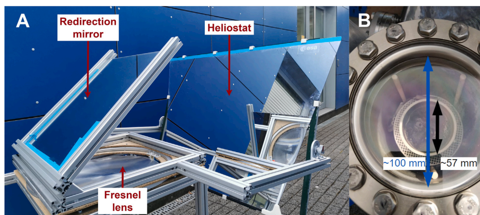
Fig. 2. Optical system of two mirrors and a Fresnel lens on the left; window of the vacuum chamber on the right.
