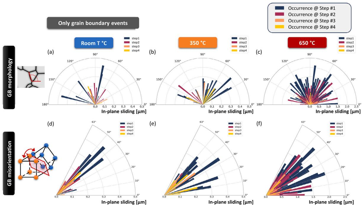
**Fig. 14.** Influence of the grain boundary morphological orientation on the onset and intensity of grain boundary sliding at (a) RT, (b) 350 °C, (c) 650 °C. Influence of the grain misorientation, *i.e.*, the crystallographic configuration, on the onset and intensity of grain boundary sliding at (a) RT, (b) 350 °C, (c) 650 °C. (For interpretation of the references to color in this figure legend, the reader is referred to the web version of this article.)
