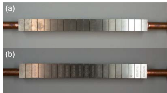
Fig. 5. Medium-scale W monoblock-type PFC mock-up with W fibre-reinforced Cu heat sink pipe. 20 W monoblocks with a plasma facing size of 12 \text{ mm} \times 23 \text{ mm} and a height of 28 mm brazed onto a 400 mm long W_t/\text{Cu} cooling pipe. The waist in the middle of the mock-up is a photographic effect and not real.
