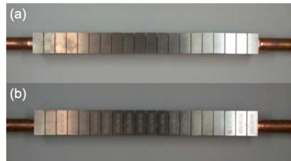
**Fig. 5.** Medium-scale W monoblock-type PFC mock-up with W fibre-reinforced Cu heat sink pipe. 20 W monoblocks with a plasma facing size of  $12 \text{ mm} \times 23 \text{ mm}$  and a height of 28 mm brazed onto a 400 mm long W<sub>f</sub>/Cu cooling pipe. The waist in the middle of the mock-up is a photographic effect and not real.
