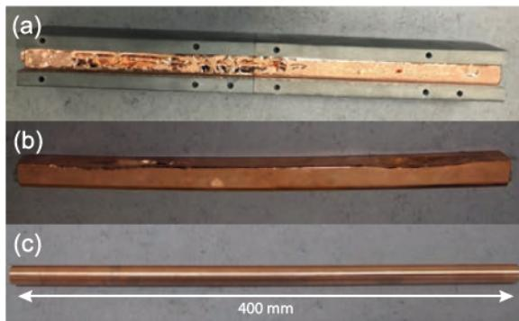
**Fig. 3.** Fabrication steps of medium-scale W fibre-reinforced Cu heat sink pipe specimen with a length of ca. 400 mm. (a) shows the Cu infiltrated W fibre braiding in mould after the casting. (b) shows the cast without mould. Cooling leads to deformation. In (c) the machined pipe is shown (outer diameter 15 mm, wall thickness 1.5 mm).
