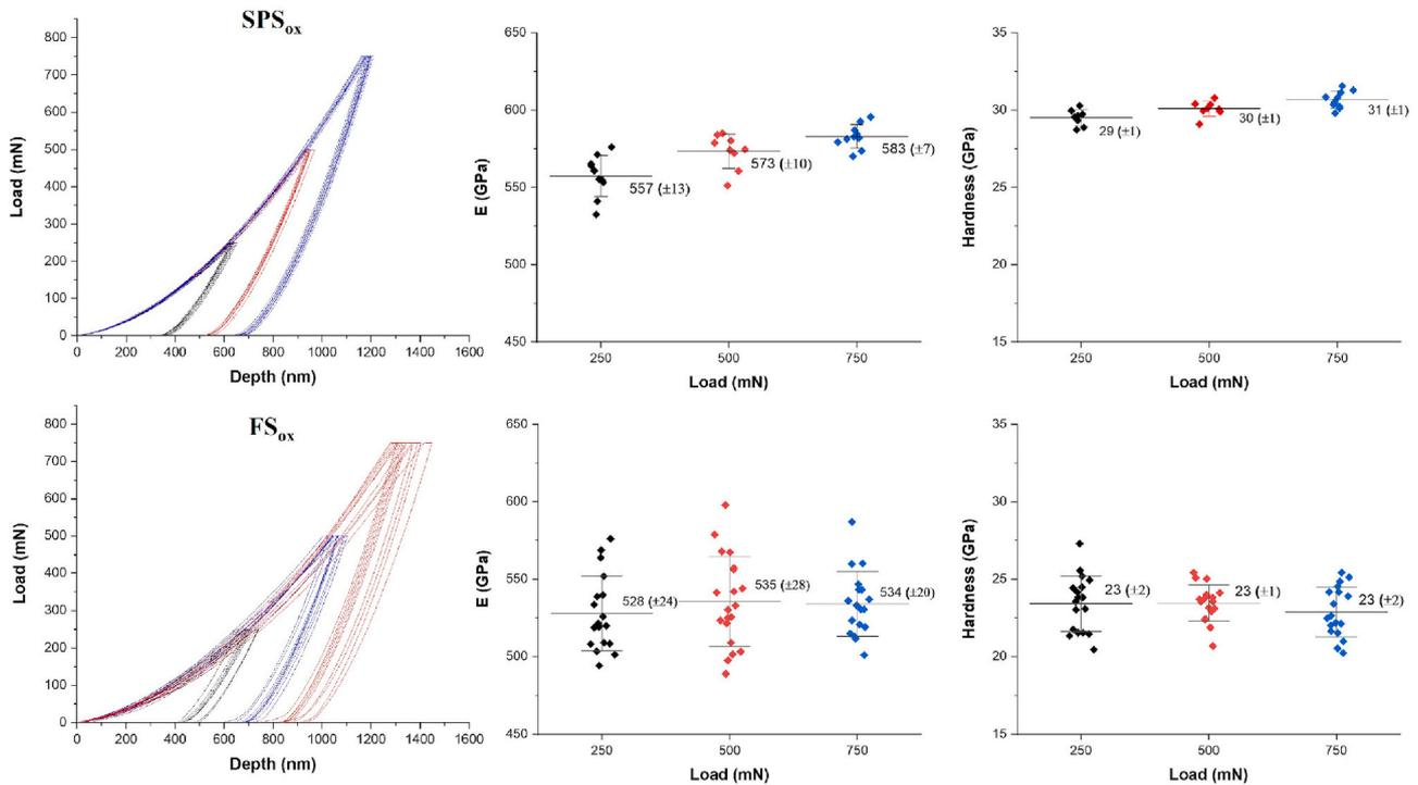
Fig. 4. Nanoindentation curves, modulus (specimen modulus  $E_s$ ) and hardness for SPS<sub>ox</sub> and FS<sub>ox</sub> samples for maximum indentation loads of 250, 500 and 750 mN.
