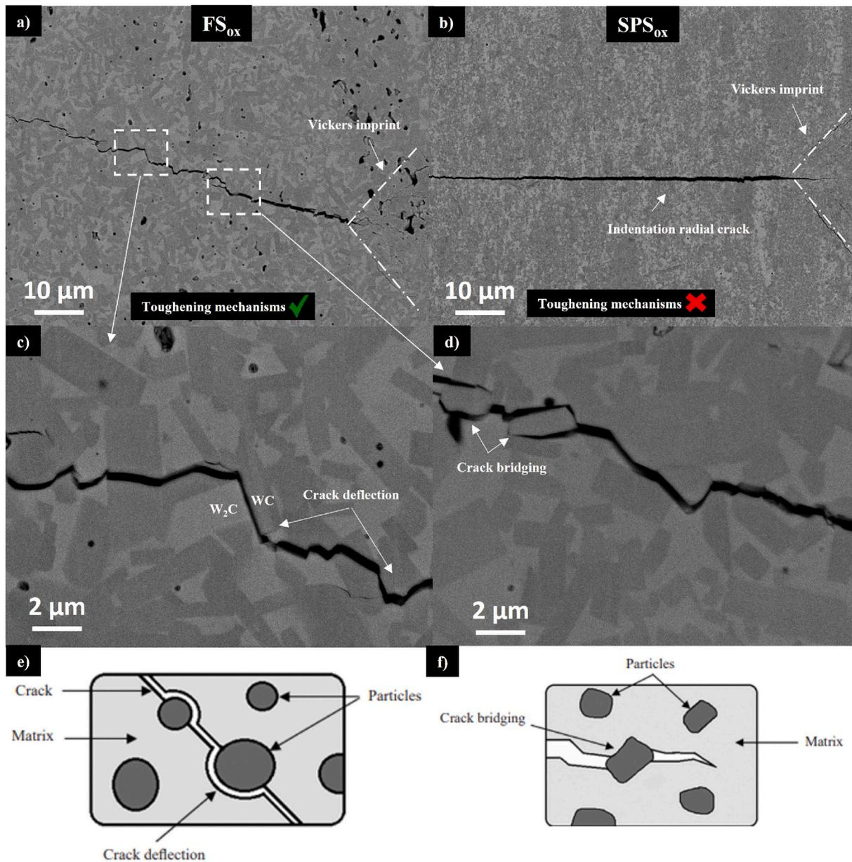
Fig. 10. Comparison of the radial crack morphology after 10 N Vickers indentation for FS<sub>ox</sub> (a) and SPS<sub>ox</sub> (b) samples. Crack deflection (c, e) and crack bridging (d, f) toughening mechanisms are active in the FS<sub>ox</sub> material thanks to the presence of elongated WC grains in a WC/W<sub>2</sub>C biphasic microstructure.
