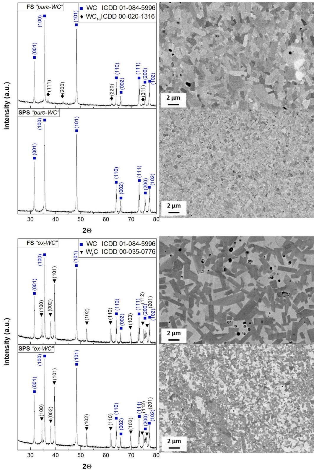
Fig. 1. Phase composition (XRD) and microstructure (FESEM-BSE) of the FS<sub>ox</sub>, FS<sub>pure</sub>, SPS<sub>ox</sub> and SPS<sub>pure</sub> samples.
