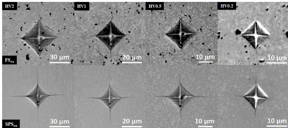
Fig. 9. Vickers indentations for FS<sub>ox</sub> (top) and SPS<sub>ox</sub> (bottom) at different maximum loads.
