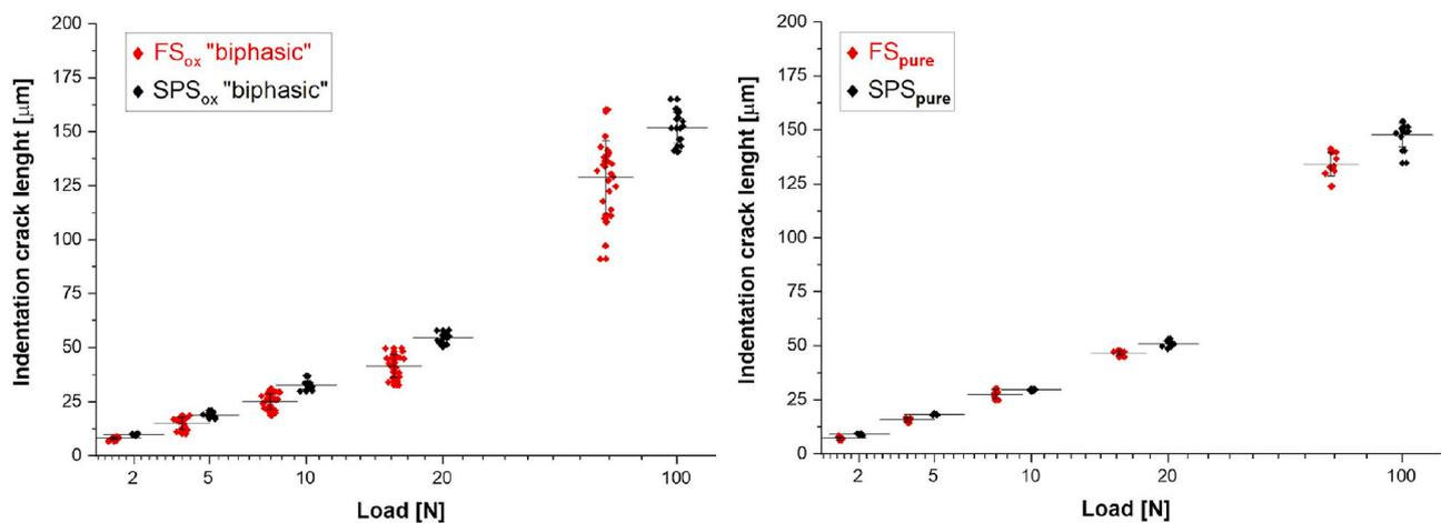
Fig. 12. Comparison of the indentation crack lengths in FS and SPS samples. The red dots are slightly shifted on the x-axis ( $\log_{10}$ ) for a representative purpose. (For interpretation of the references to colour in this figure legend, the reader is referred to the Web version of this article.)
