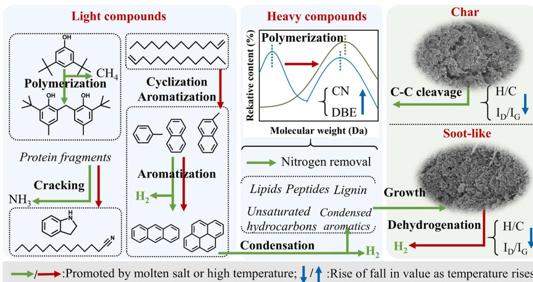
Fig. 8. Transformation pathways of pyrolysis products in molten NaOH-Na<sub>2</sub>CO<sub>3</sub>.
