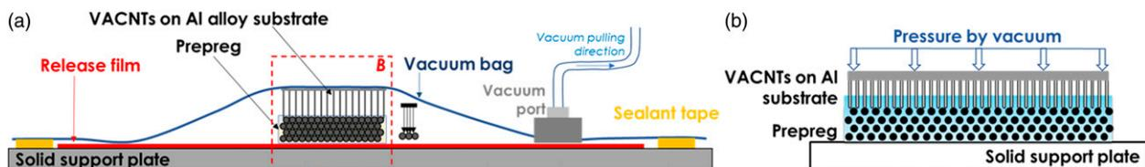
**Figure 3.** Vacuum impregnation process: a piece of prepreg and an Al alloy growth substrate with the synthesised VACNTs placed on the prepreg' top are placed under a vacuum bag to distribute pressure evenly across the VACNTs-prepreg contact surface.
