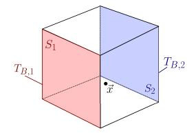
Figure 9: Schemes of the solid cube with two isothermal faces  $S_1$  and  $S_2$ , respectively at temperature  $T_{B,1}$  and  $T_{B,2}$ , with a location  $\vec{x}$  inside the solid volume.
