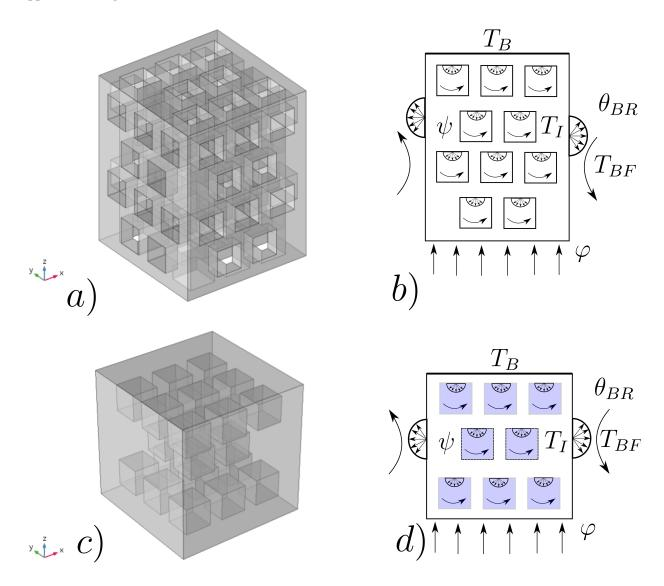
Figure C.13: Schemes of the two benchmark configurations. **a**) Geometry with open cavities; **b**) Different sources applied to this first benchmark for the physical problem. - **c**) Geometry with enclosed cavities; **d**) Sources applied the second benchmark for the physical problem.
