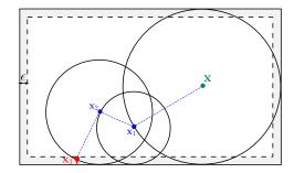
Figure 4: Illustration of the sampling of a random path using the random walk-on-sphere method to estimate density at location **x**. In order to end the random walk, the boundary of the domain is thickened of a small value  $\epsilon$  in which the final position **x**<sub>3</sub> is projected on the boundary.
