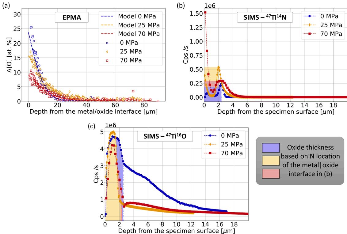
Fig. 1. EPMA (a), SIMS for  $^{47}\text{Ti}^{14}\text{N}$  (b) and  $^{47}\text{Ti}^{16}\text{O}$  experimental data(c). Fitting of EPMA results are also plotted in (a). Depth data for  $^{47}\text{Ti}^{16}\text{O}$  were re-adjusted by using the position of the maxima for  $^{47}\text{Ti}^{14}\text{N}$ .
