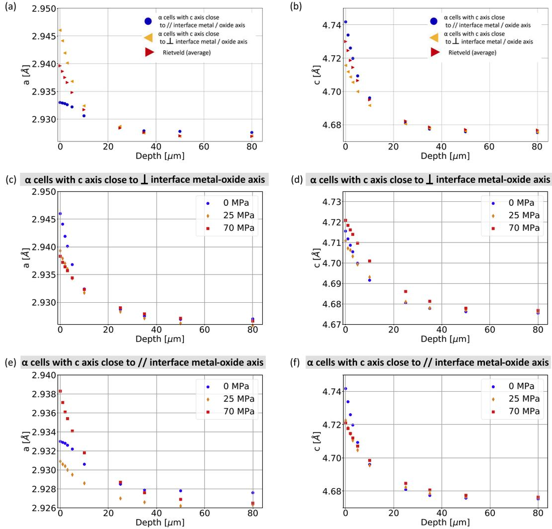
Fig. 4. Comparison of peak by peak and Rietveld methods on parameters  $a$  (a) and  $c$  (b) for unloaded sample. Influence of tensile stress on peak by peak results considering different  $\alpha$ -cell populations for parameters  $a$  (c & e) and  $c$  (d & f).
