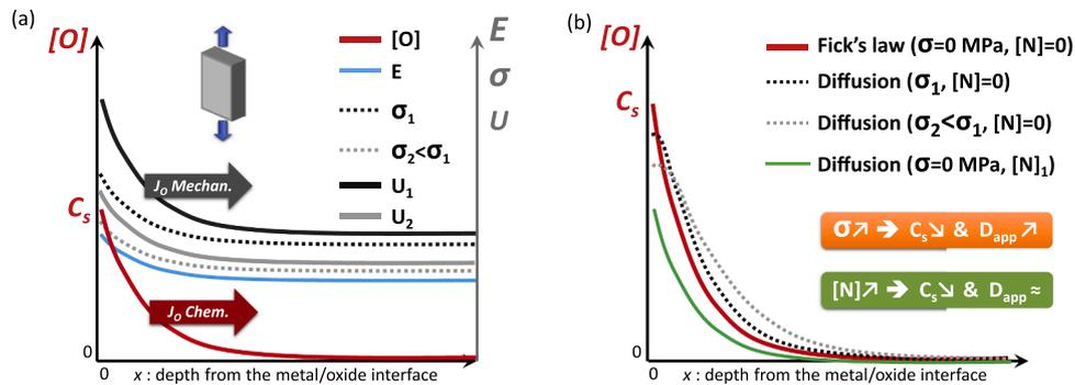
Fig. 5. Schematic illustration of oxygen profile, elastic energy  $U$ , Young modulus  $E$  and stress level  $\sigma$  within ORL (a) and how oxygen profile can be influenced by nitrogen presence and/or load application (b).
