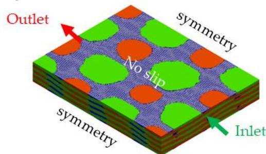
Figure 2. Simulation geometry and boundary conditions.
