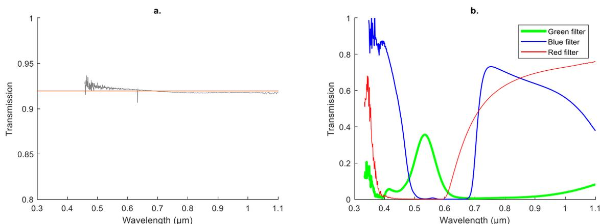
**Fig. 3.** (a.) Transmission spectrum at room temperature of the furnace glass windows and (b.) transmission spectrum at room temperature of the green, blue and red filters. (For interpretation of the references to colour in this figure legend, the reader is referred to the Web version of this article.)
