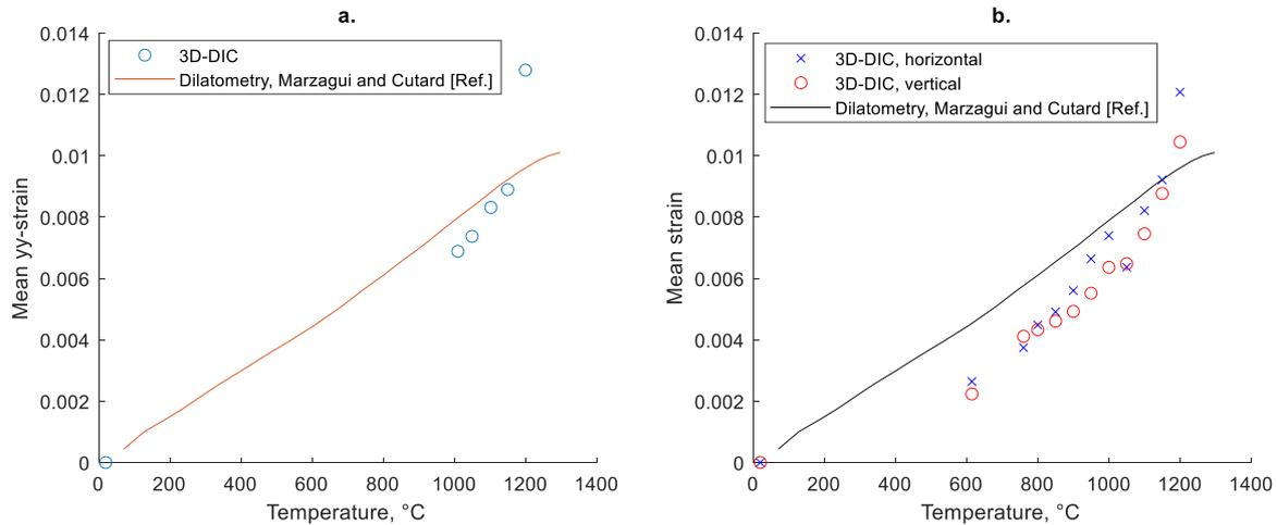
**Fig. 16.** Thermal expansion strain of (a.) a cylindrical sample (vertical axial strain) and (b.) of the flat surface of a parallelepipedal sample (in horizontal and vertical directions), measured by 3D-DIC from room temperature up to 1200 °C, compared to the dilatometric curve in Ref. [24] (same refractory concrete, but unreinforced by metallic fibres). A large part of the gap is related to the different thermal management and sample volume in both experiments.
