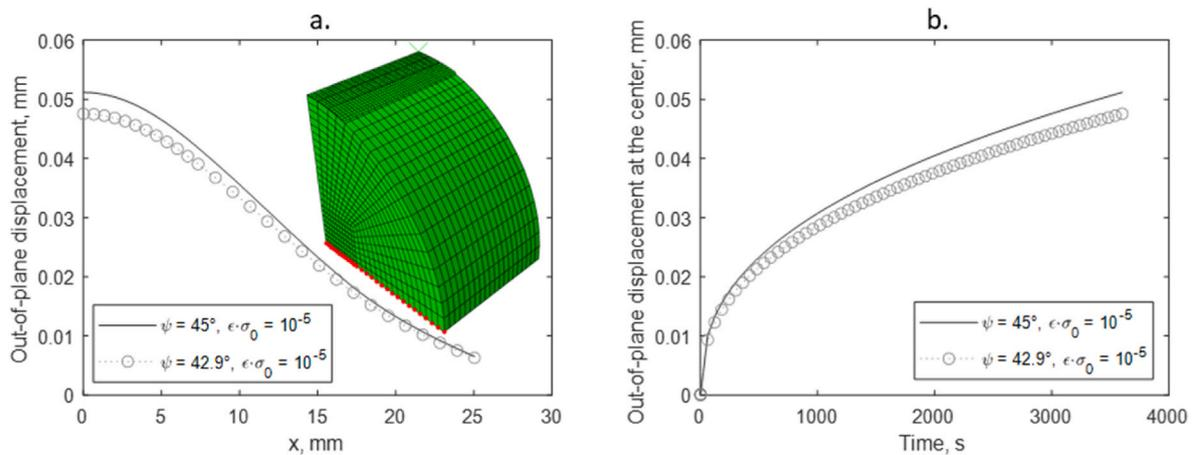
**Fig. 14.** Out-of-plane displacement after 1 h creep at 1200 °C in diametral compression along the horizontal axis at the surface of the specimen (a.) and out-of-plane displacement as a function of time at the centre of the specimen assuming to values of dilation angle (b.). Eccentricity  $\epsilon \bullet \bar{\sigma}_0$  in MPa.
