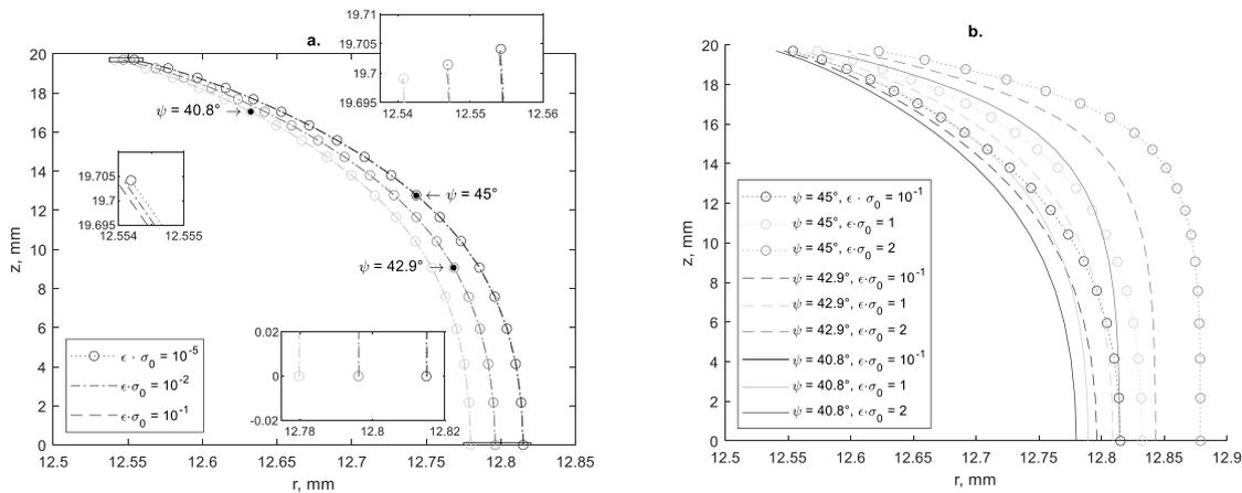
Fig. 10. Profile of the compression sample computed for several values of dilation angle  $\psi$  and eccentricity  $\epsilon \cdot \bar{\sigma}_0$  (in MPa) (a.) for low eccentricity values and (b.) for high eccentricity values.
