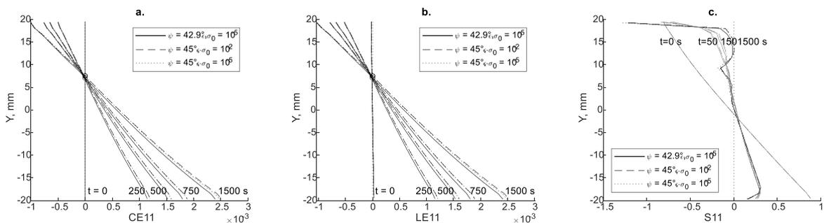
Fig. 12. (a.) creep strain CE11 (b.) total strain LE11 and (c.) stress S11, in the length-wise direction of the sample at several times and computed for several values of dilation angle  $\psi$  and eccentricity  $\epsilon \cdot \bar{\sigma}_0$  (in MPa).
