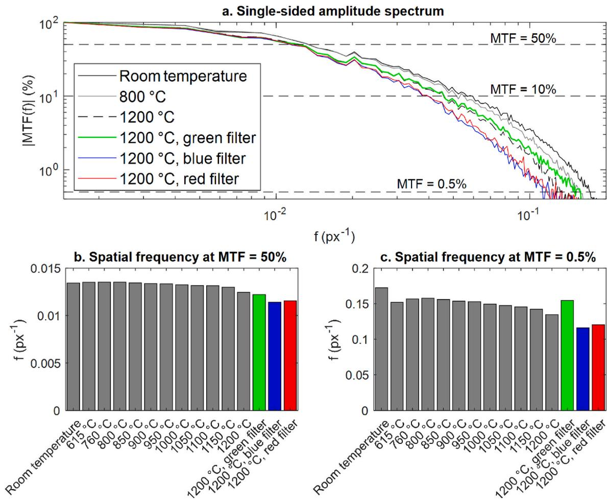
**Fig. 8.** Single sided amplitude spectrum (a.) and spatial frequency at 50 % (b.) and 0.5 % (c.) amplitude as a function of temperature without filter, and with a green, blue or red filter at 1200 °C. (For interpretation of the references to colour in this figure legend, the reader is referred to the Web version of this article.)
