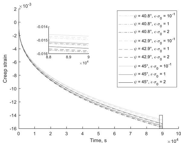
**Fig. 9.** Creep deformation during compression test at 1200 °C computed with different values of dilation angle,  $\psi$  and eccentricity  $\epsilon \cdot \bar{\sigma}_0$  (in MPa).
