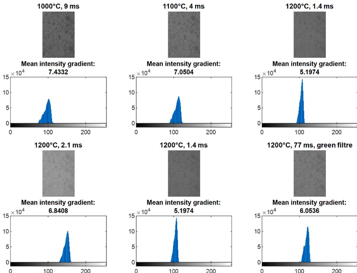
**Fig. 7.** Effect of temperature, integration time and green filter on MIG of mean images. (For interpretation of the references to colour in this figure legend, the reader is referred to the Web version of this article.)
