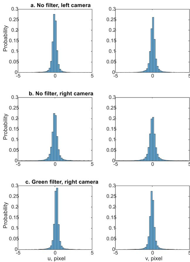
**Fig. 5.** Typical horizontal (u) and vertical (v) displacements histogram (a.) without any filter, left camera (integration time 1.4 ms), (b.) without any filter, right camera (integration time 1.4 ms) and (c.) with the green filter, right camera (integration time 68 ms). (For interpretation of the references to colour in this figure legend, the reader is referred to the Web version of this article.)
