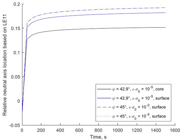
**Fig. 13.** Relative vertical location of the neutral axis based on LE11 ( $\frac{y_{LE11=0}}{h}$ ), with the y-origin in the mid-height of the sample, at the surface and at core of the sample, as a function of time for several values of dilation angle  $\psi$  and eccentricity  $\epsilon \bullet \bar{\sigma}_0$  (in MPa).
