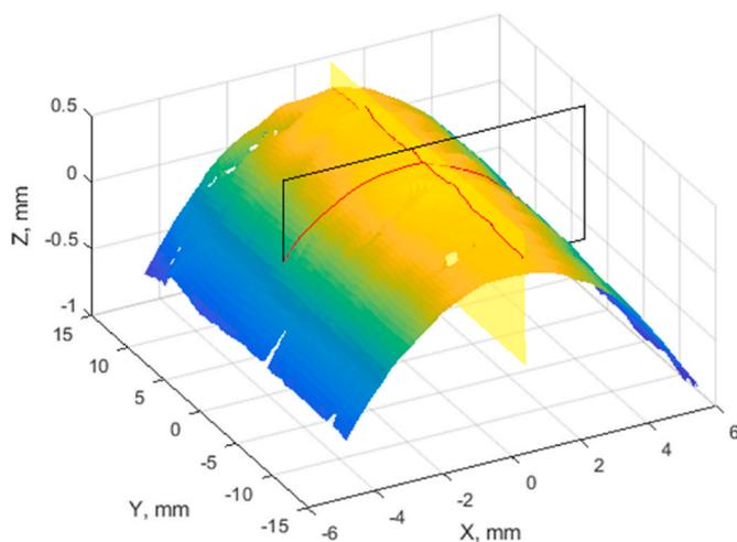
**Fig. 17.** Surface measured by 3D-DIC on a cylindrical sample at 1200 °C. The red lines are the profiles extracted to perform curvature analysis (Figs. 18 and 19). (For interpretation of the references to colour in this figure legend, the reader is referred to the Web version of this article.)
