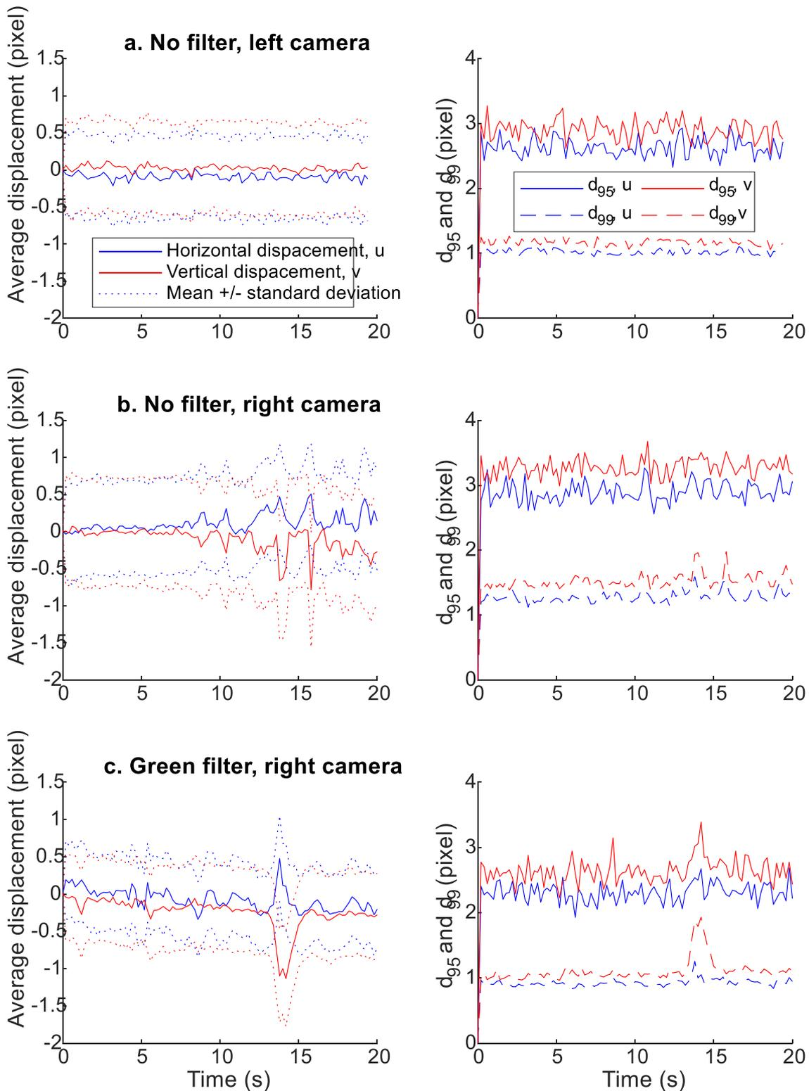
**Fig. 6.** Average displacement as a function of time (left), and 95th and 99th percentiles,  $d_{95}$  and  $d_{99}$  (right); without any filter (integration time 1.4 ms) (a. and b.), with green filter (integration time 68 ms) (c.), left camera (a.) and right camera (b. and c.). (For interpretation of the references to colour in this figure legend, the reader is referred to the Web version of this article.)
