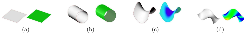
Figure 6: Surface approximation for virtual model creation: (a) simple planar surface, (b) simple curved surface, (c) complex curved surface, (d) Complex free-form surface.
