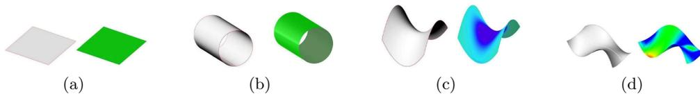
Figure 6: Surface approximation for virtual model creation: (a) simple planar surface, (b) simple curved surface, (c) complex curved surface, (d) Complex free-form surface.
