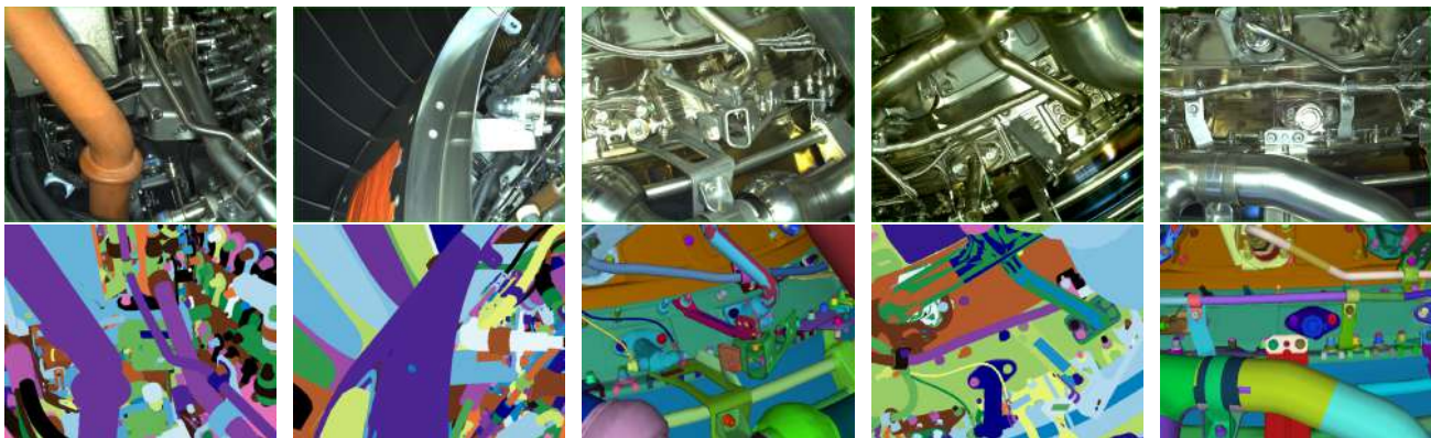
Figure 4: The first row represents the 2D images taken by the camera with a wide field of view. The second row represents the synthetic renderings corresponding respectively to the image acquisitions from the first row.
