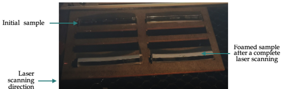
Figure 2. Laser foaming experimental setup with inserted samples.
