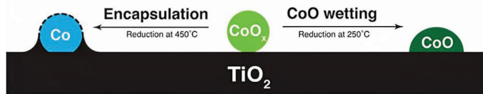
Figure 6. Metallic Co encapsulation and CoO wetting over TiO 2 after reduction at 450 and 250 °C, respectively. Reproduced with permission. [33] Copyright 2014, American Chemical Society.
