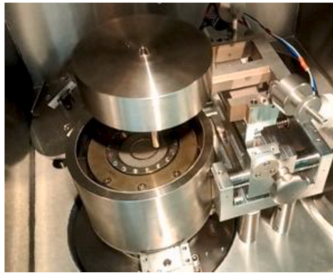
Fig. 2. Side view of the ball-on-disc type CSM Instruments tribometer.
