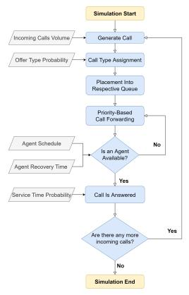
Figure 4: Simulation flow chart.
