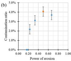
Fig. 11. Position of the delaminated plies (a) and contamination ratio (b) as a function of the "power of erosion".
