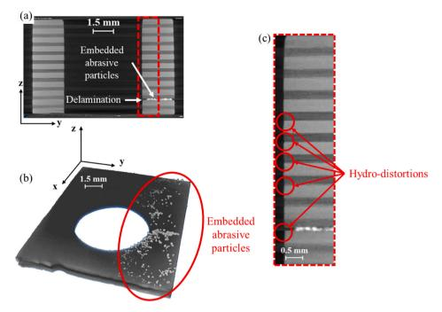
Fig. 9. Tomography pictures showing delamination (a), grit contamination (b) and hydro-distortions through the thickness of the GLARE plate (c) induced by AWJ drilling.
