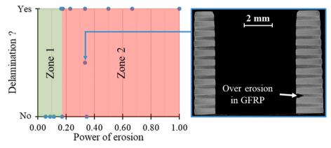
Fig. 10. Delamination with respect to the "power of erosion" of the AWJ drilling operation.
