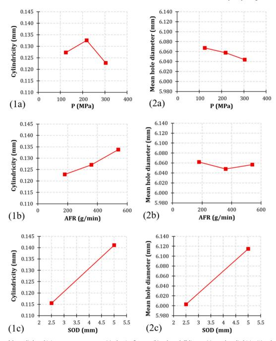
Fig. 3. Influence of the studied machining parameters – pressure (a), abrasive flow rate (b) and standoff distance (c) – on the cylindricity (1) and mean diameter (2) of the holes.
