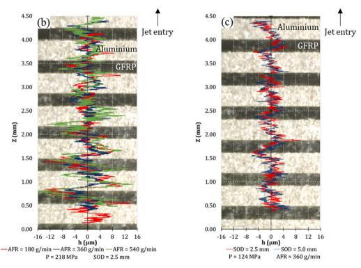
Fig. 7. Evolution of the profiles measured by the surface roughness tester in 90° direction as a function of (a) the jet pressure, (b) the abrasive flow rate and (c) the standoff distance.
