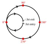
**Fig. 2.** Cutting path strategy used in this study. The four orientations correspond to the roughness measurements.
