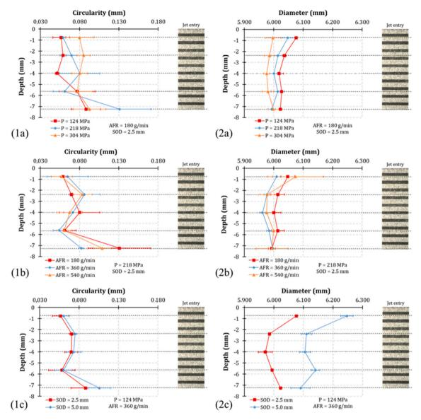
Fig. 4. Influence of the studied machining parameters – water pressure (a), abrasive flow rate (b) and standoff distance (c) – on the circularity (1) and diameter (2) of different circles probed along the holes.
