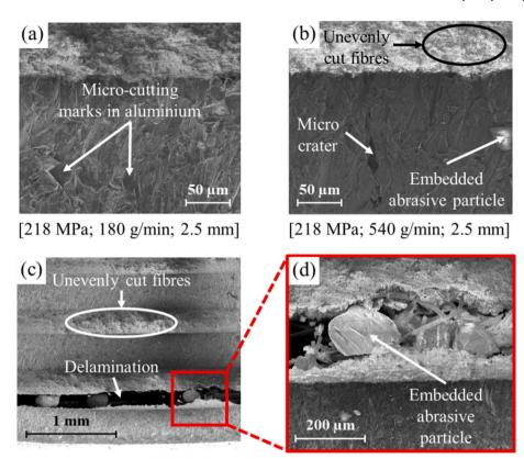
Fig. 8. SEM pictures showing the defects induced by AWJ drilling on GLARE with: (a) micro-cutting marks, (b) micro-craters and embedded particles in aluminium, (c, d) unevenly cut fibres in GFRP and delamination with embedded abrasive particles at the interface.
