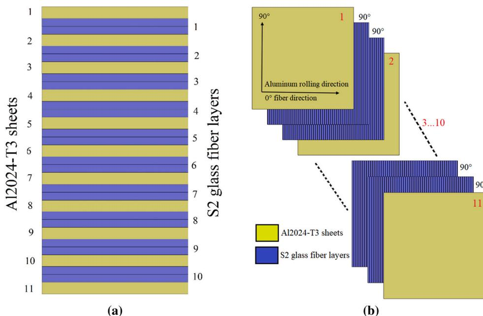
Fig. 1. GLARE workpiece details (a) side view (b) constituents order.
