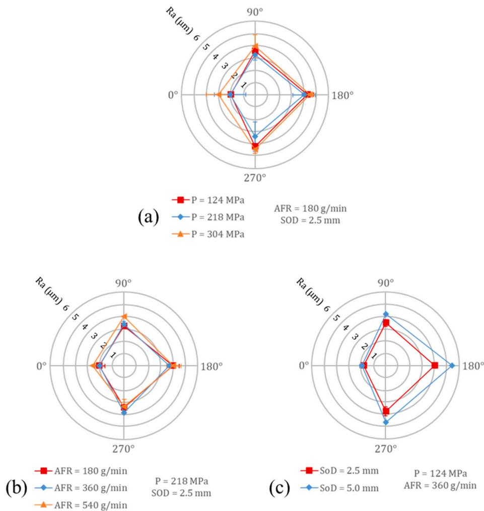
Fig. 6. Influence of the studied machining parameters – pressure (a), abrasive flow rate (b) and standoff distance (c) – on the mean arithmetic surface roughness (Ra) of the holes in four directions. 0° corresponds to both the jet entry and exit.
