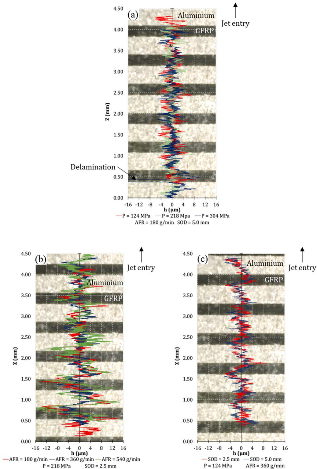
Fig. 7. Evolution of the profiles measured by the surface roughness tester in 90° direction as a function of (a) the jet pressure, (b) the abrasive flow rate and (c) the standoff distance.
