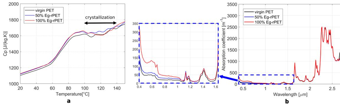
**Figure 2.** Properties of materials used (a) Specific heat capacity and (b) Absorption coefficient.
