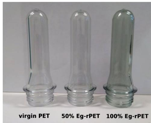
**Figure 1.** Preforms made from different materials.
