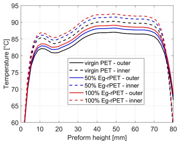
**Figure 7.** Simulated temperature profile along the preform height of different material grades.
