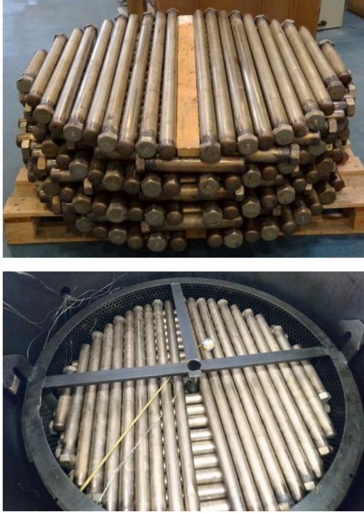
Fig. 9. The final PCM layer package.
