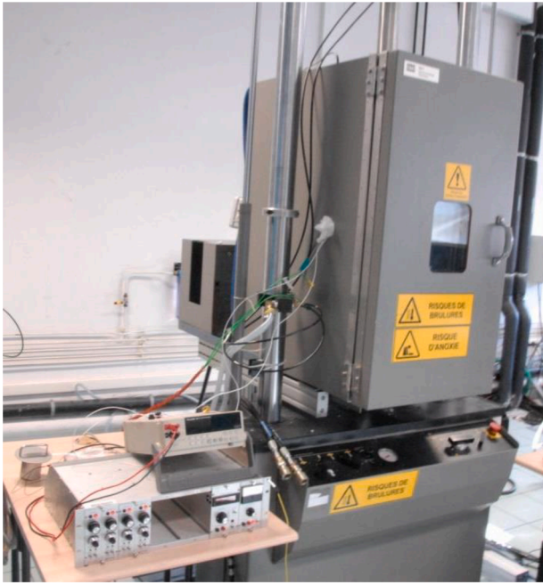
Fig. 4. Experimental setup for monotonic, loading/unloading traction tests.
