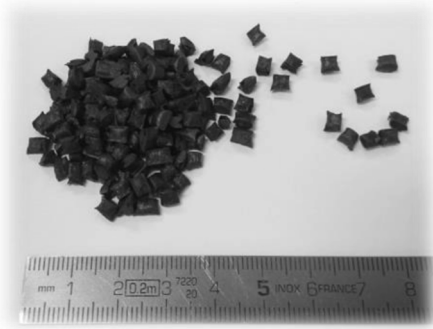
Fig. 1. Pellets of Victrex® PEEK 90HMF40.
