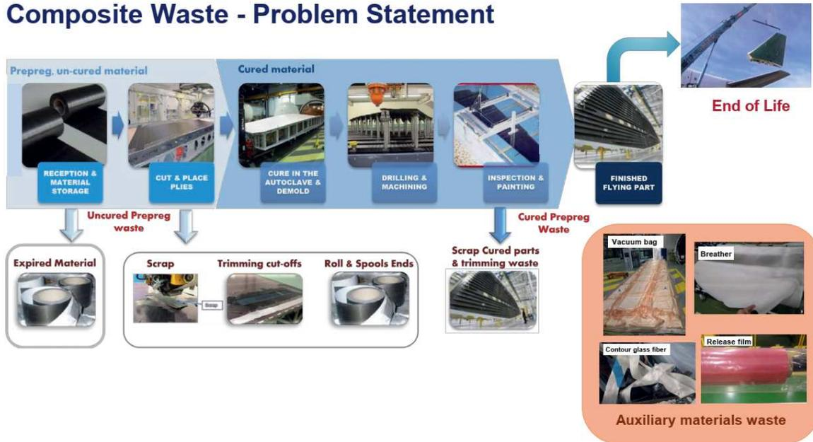
FIGURE 6: SOURCES DE DÉCHETS COMPOSITES DANS L'AÉRONAUTIQUE. [14]
