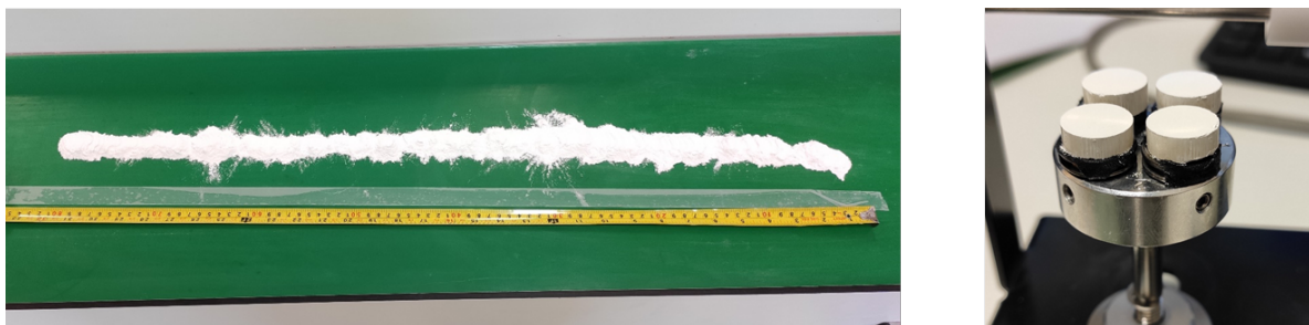
Figure 5: Ground powder spread out for the sampling procedure (left) and pellets obtained after compacting (right)
