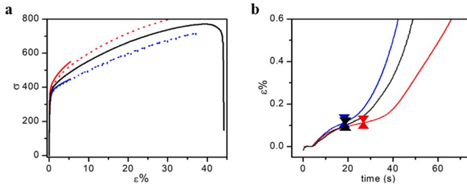
**Fig. 9.** a) Tensile curves of cylindrical hybrid treated samples (black) equipped with local gauges on the DED (blue) and LPBF (red) zones, compared to global full DED and LPBF treated samples (dashed). b) Measurements by the global extensometer (black) and local gauges (red/blue) relative to the testing time. (For interpretation of the references to colour in this figure legend, the reader is referred to the web version of this article.)
