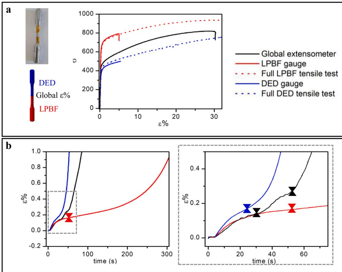
**Fig. 8.** a) Tensile curves of a cylindrical hybrid sample (black) equipped with local gauges on the DED (blue) and LPBF (red) zones, compared to full DED and LPBF samples (dashed). b) Measurements by the global extensometer (black) and local gauges (red/blue) relative to the testing time. (For interpretation of the references to colour in this figure legend, the reader is referred to the web version of this article.)
