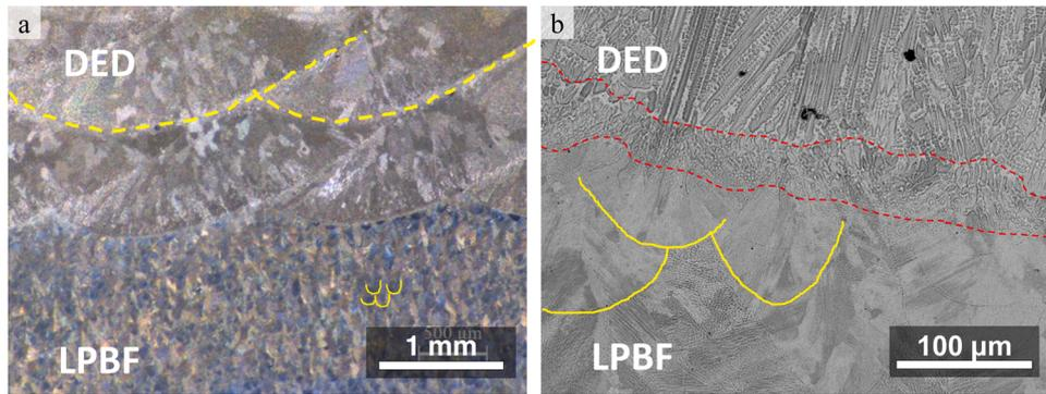
Fig. 3. a) Optical and b) SEM observations of hybrid LPBF - DED Inconel 625. (For interpretation of the references to colour in this figure, the reader is referred to the web version of this article)
