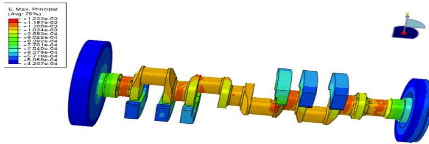
Fig. 5. Equivalent principal strain state on the crankshaft
