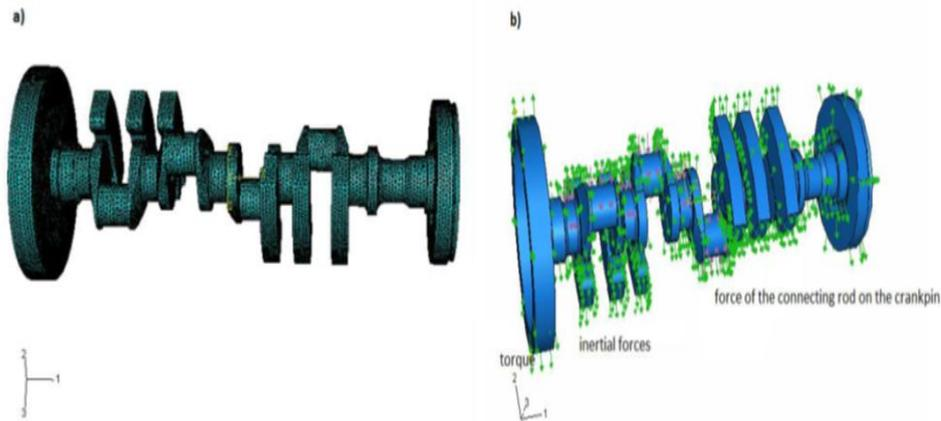
Fig. 2. Crankshaft modelling: a) Mesh, b) applied loads
