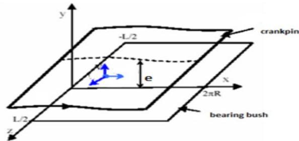
Fig. 1. Calculation scheme for convection coefficients [12]
