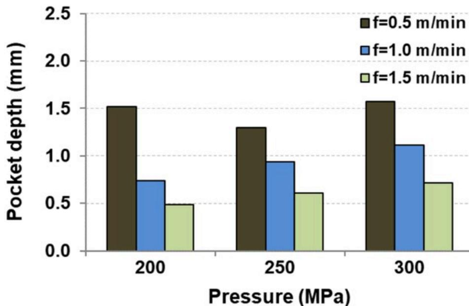
Fig. 4. Effect of pressure and traverse speed on pocket depth.
