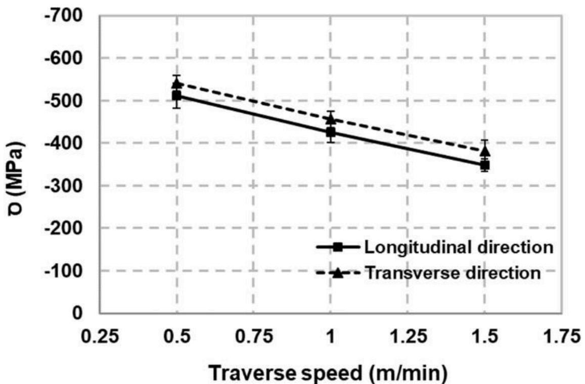
Fig. 5. Effect of traverse speed on residual stresses.
