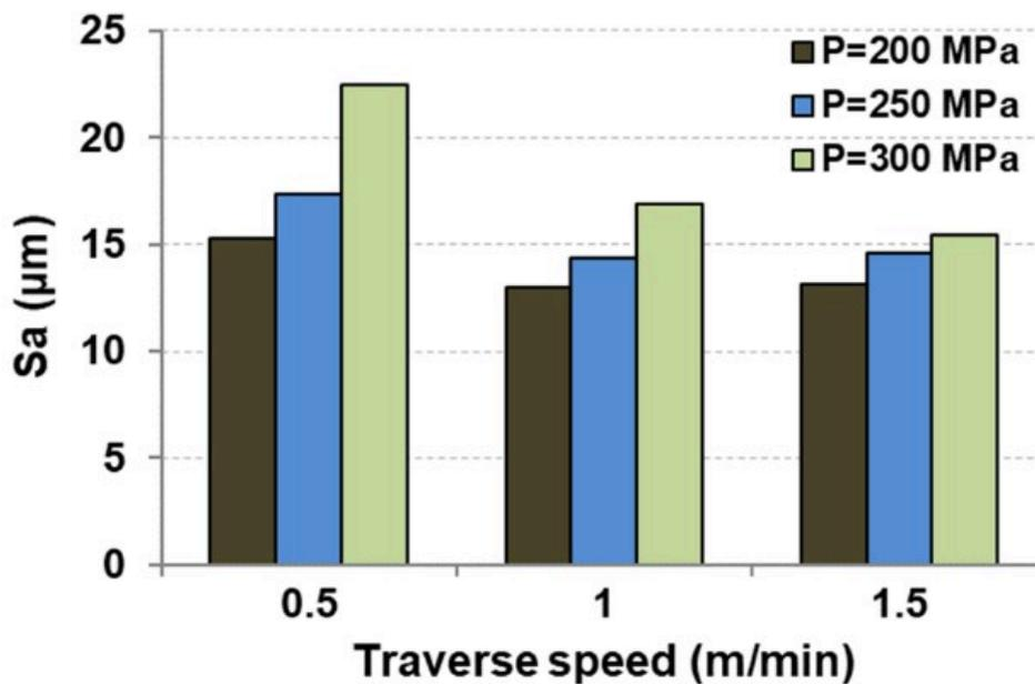
Fig. 2. Effect of pressure and traverse speed on surface roughness.
