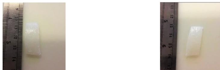
Figure 3. Nodule pieces after 7 days ( left ) and 28 days ( right ) in contact with the SA–PA mixture at 85 °C.
