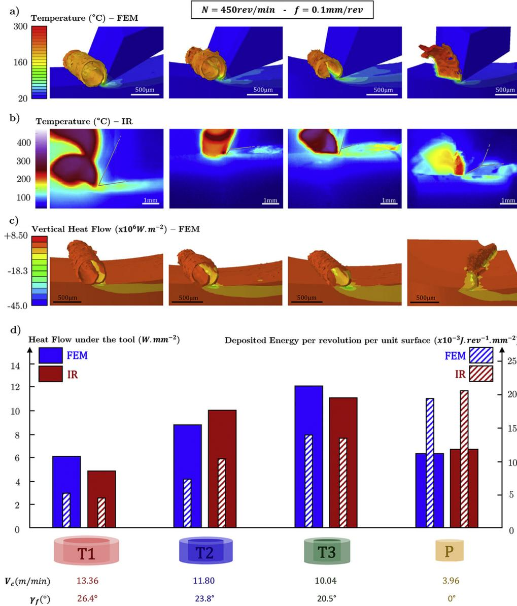
**Fig. 15.** Thermal results on the 1st revolutions for a spindle speed  $N=450 \text{ rev/min}$  and a feed rate  $f=0.1 \text{ mm/rev}$  – (a) FEM Temperature (b) IR Temperature (c) FEM Vertical Heat Flow (d) Heat Flow under the tool and deposited energy per rev per unit of the workpiece surface ( $50 \mu\text{m} \times 50 \mu\text{m}$ ) – for every local cutting speed  $V_c$  and local rake angle  $\gamma_f$ .
