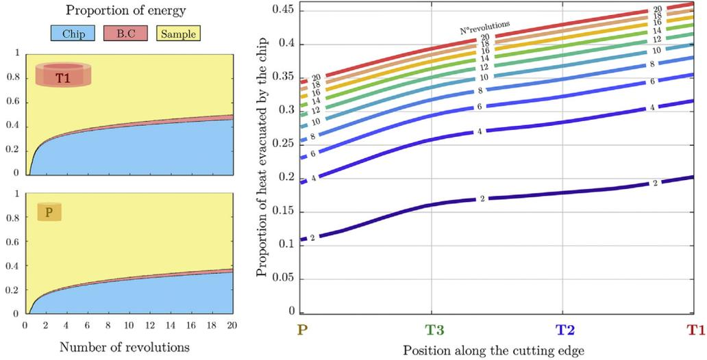
**Fig. 20.** Numerical prediction of the energy budget (a) time evolution of the part of energy that enters the material and that ultimately remain in it (yellow), is drains off latter by the chip (blue), and lost to the environment (red) – (b) Radius wise representation of the energy budget (time evolution).
