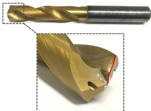
Fig. 2. SECO-SD203A-11.0-33-12R1-M twist drill used in the experiment.
