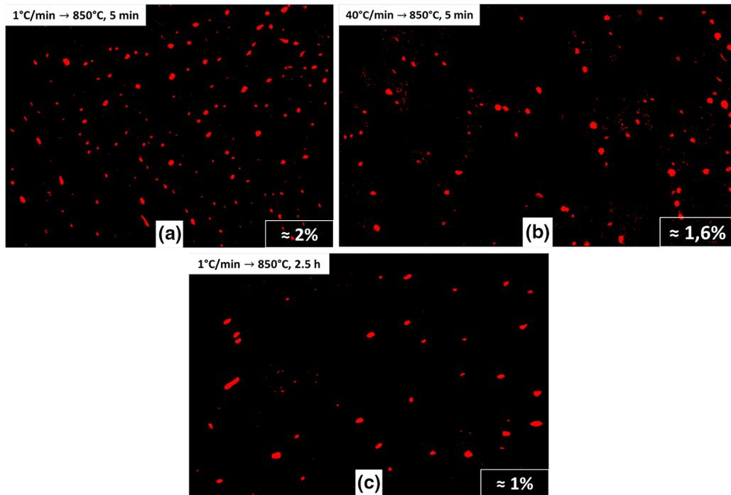
Fig. 10—Image analysis based on the STEM-EDX maps presented in Figs. 8(a) through (c). The  $\beta$ -NiAl precipitates from the thresholding process appear in red and the surface fractions estimated are indicated at the bottom right of each image (Color figure online).
