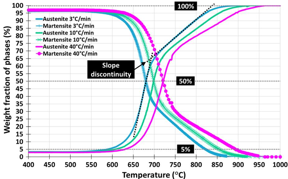
Fig. 7—Evolution of martensite and austenite weight fractions quantified by Rietveld refinement according to temperature between 400 °C and 1000 °C at 3, 10 or 40 °C/min heating rates.
