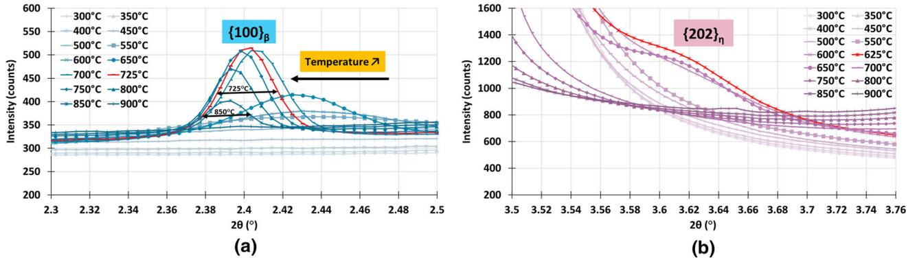
Fig. 6—Evolution of the (a)  $\{100\}_\beta$  and (b)  $\{202\}_\eta$  diffraction peaks every 50 °C between 300 °C and 900 °C during heating at 3 °C/min. FWHM are indicated in figure (a) for temperatures of 725 °C and 850 °C.
