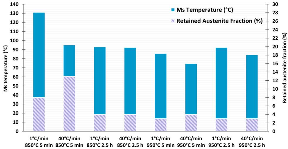
Fig. 9— $M_s$  temperature and retained austenite fraction estimated for different austenitization conditions during a 5 °C/min cooling by dilatometry and after quenching by XRD, respectively. The austenite and martensite phase fractions were quantified in this case using the Reference Intensity Ratio (RIR) method. The RIR method is carefully described in Ref. [38].
