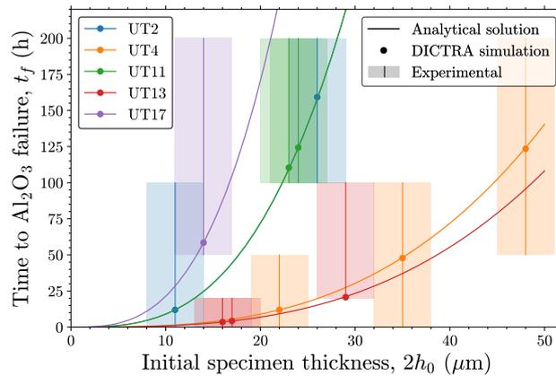
**Figure 17:** Time to  $\text{Al}_2\text{O}_3$  failure determined from the DICTRA simulations and the analytical solution, Eq. (11). Experimental values are also given, as intervals determined by visually inspecting the specimens at each interruption. The shaded rectangles are defined by these intervals and a  $\pm 3 \mu\text{m}$  range around the average initial specimen thickness.
