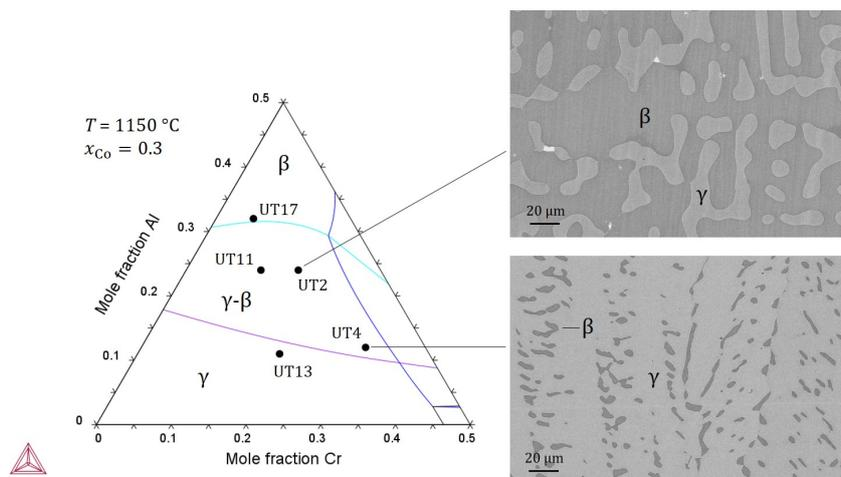
**Figure 1:** Nominal alloy compositions projected on an isothermal, isoplethal section ( $T = 1150\text{ °C}$ ,  $x_{\text{Co}} = 0.3$ ) of the NiCoCrAl phase diagram, calculated with Thermo-Calc [24] and the CRALDAD database [26, 27]. Note that not all alloys are on the  $x_{\text{Co}} = 0.3$  isopleth. SEM micrographs showing the bulk microstructure of 2-phase alloys are also included.
