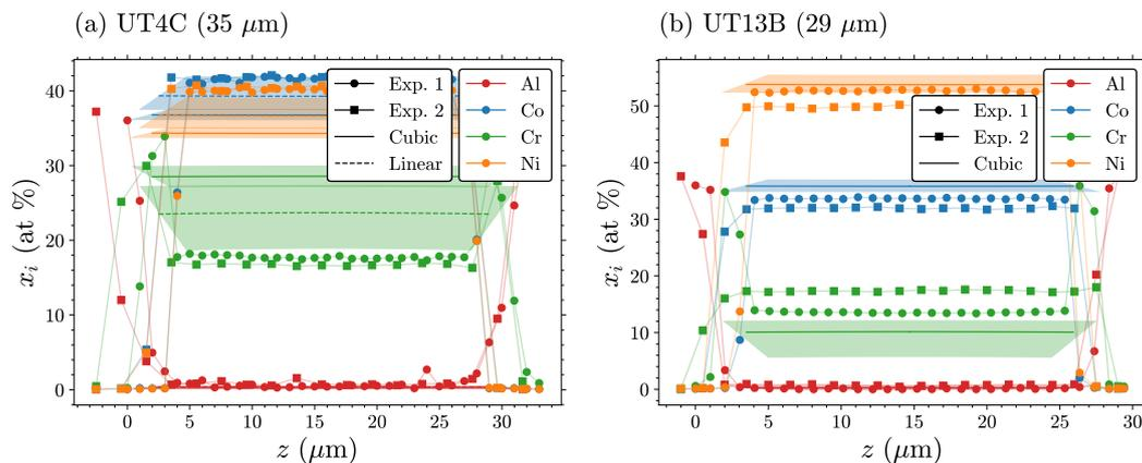
**Figure 13:** Experimental and simulated (DICTRA) concentration profiles for alloys (a) UT4C and (b) UT13B after 200 h at 1150 °C. Simulated profiles obtained with either cubic or linear  $\text{Cr}_2\text{O}_3$  growth kinetics — see text for details. In (b), linear kinetics led to full Cr consumption before the end of the 200 h simulation.
