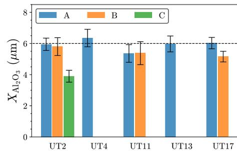
**Figure 7:** Average scale thickness measured on specimens that only formed  $\text{Al}_2\text{O}_3$ , after 200 h at 1150 °C. The dashed line shows the value corresponding to the boundary condition used in the DICTRA simulations.
