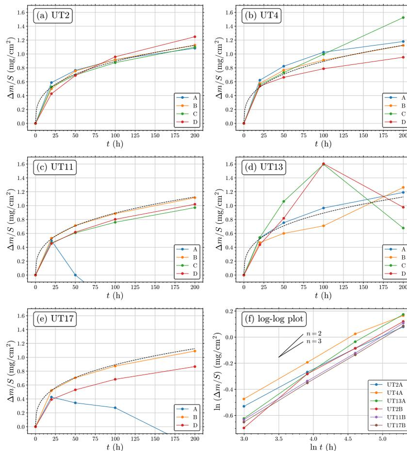
**Figure 5:** Mass changes recorded during oxidation at 1150 °C. In (a)-(e), the dashed line represents the mass gains corresponding to the growth of a pure  $\text{Al}_2\text{O}_3$  scale according to the rate law chosen for the simulations, Eq. (1) and Table 3; (f) shows a log-log plot for the specimens that remained in the stage of  $\text{Al}_2\text{O}_3$  growth throughout the 200 h.
