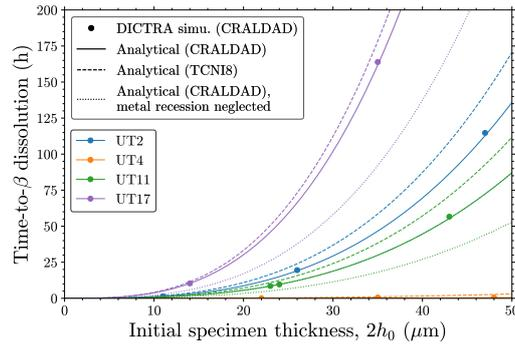
**Figure 16:** Time to  $\beta$  dissolution determined from the DICTRA simulations. Also included are the results from the analytical solution, Eq. (8), where the threshold Al fraction for  $\beta$  stability was calculated using either CRALDAD or TCNIS, and the results obtained by further neglecting the metal recession, Eq. (10) (see text for details).
