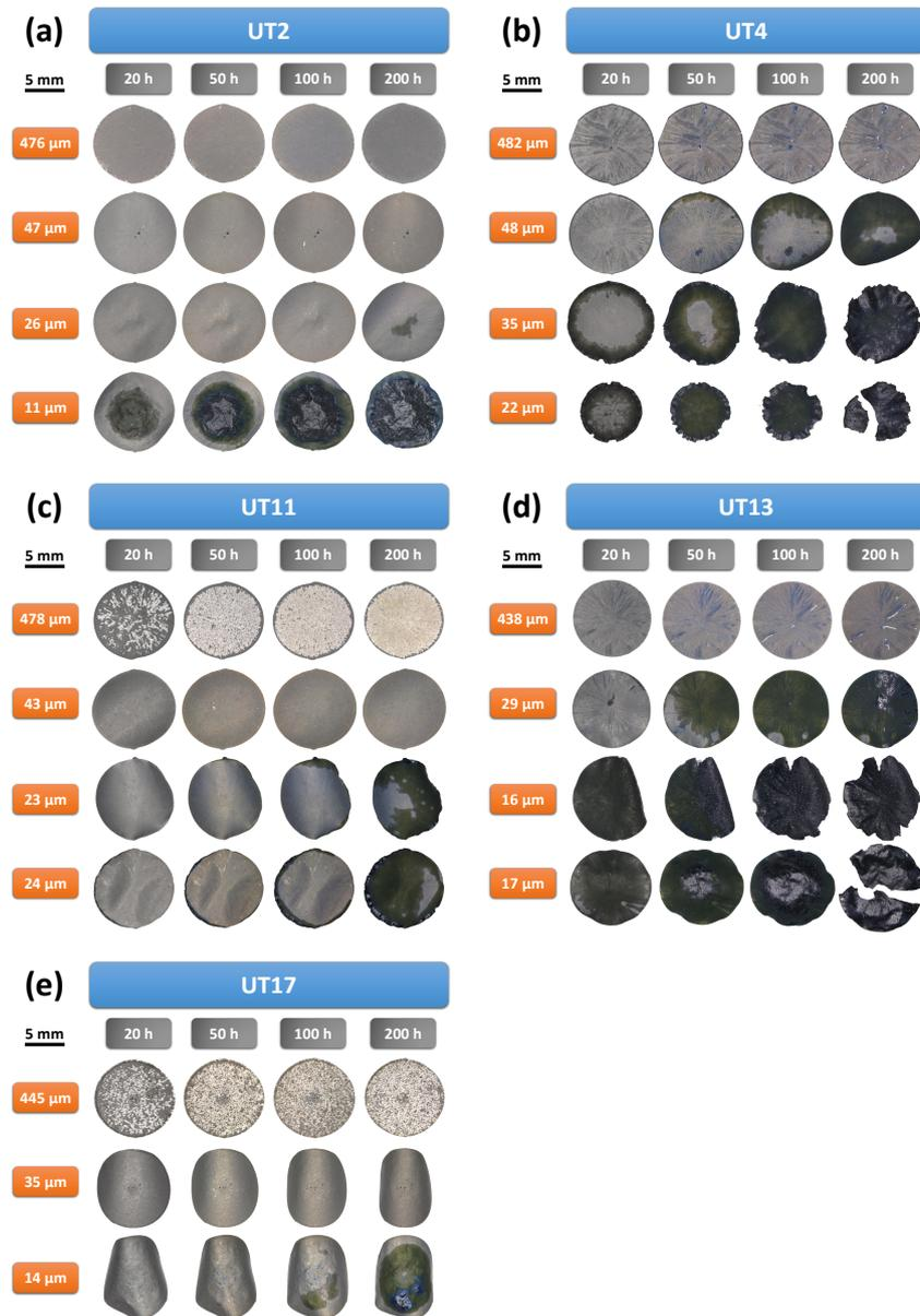
**Figure 4:** Photographs of the specimens at interruptions of the 1150 °C oxidation experiment. Grey/blue:  $\text{Al}_2\text{O}_3$ ; dark green:  $\text{Cr}_2\text{O}_3$ ; dark grey: Ni- and Co-rich oxides; light grey: alloy.
