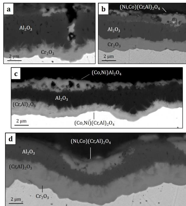
**Figure 9:** Cross-section SEM images of alloys (a) UT4B (48  $\mu\text{m}$ ), (b) UT13B (29  $\mu\text{m}$ ), (c) UT2D (11  $\mu\text{m}$ ) and (d) UT4C (35  $\mu\text{m}$ ) after 200 h oxidation at 1150  $^{\circ}\text{C}$ .
