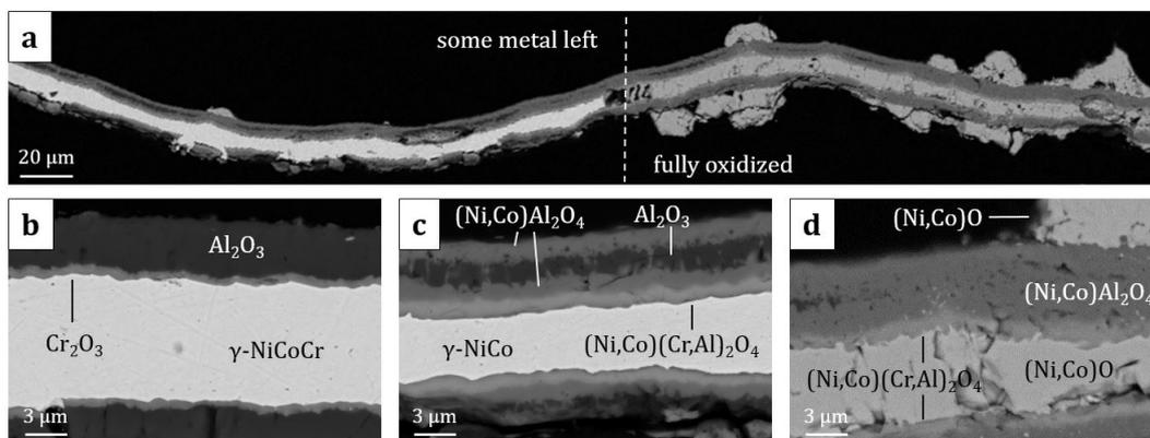
**Figure 8:** Cross-section SEM images of alloy UT17D (14 μm) after 200 h oxidation at 1150 °C, showing several stages of the oxidation process. (a) Overview, (b)  $\text{Al}_2\text{O}_3$  and thin  $\text{Cr}_2\text{O}_3$ , (c) Ni and Co oxide around the  $\text{Al}_2\text{O}_3$ , and (d) alloy fully oxidized.
