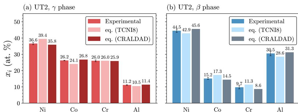
**Figure 3:** Phase compositions in  $\gamma$ - $\beta$  alloy UT2 in the as-received state (annealed at 1150 °C) measured by SEM-EDS, compared with equilibrium values at 1150 °C calculated with Thermo-Calc and the TCNI8 and CRALDAD databases. (The experimental values represent the mean of 30 point analyses. The error bars represent the standard deviation for each series.)
