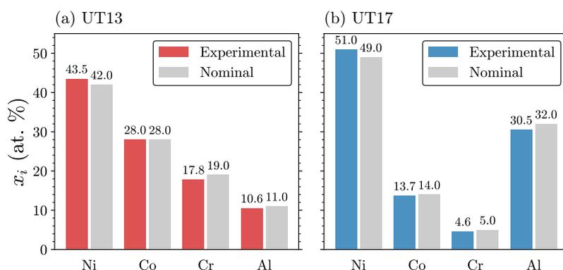
**Figure 2:** Compositions of single-phase alloys (a) UT13 ( $\gamma$ ) and (b) UT17 ( $\beta$ ) in the as-received state measured by SEM-EDS, compared with nominal compositions. (The experimental values represent the mean of 11 point analyses. The standard deviation for each series was about 0.1–0.2 at. %.)
