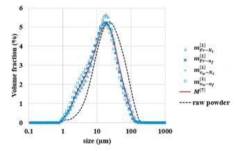
**Fig. 14.** Volume particle size distribution of the powder samples ground in the 1 L and the 7 L vessels in various conditions described in Table 7.
