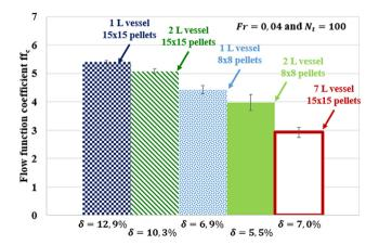
**Fig. 12.** Flow function coefficient of powder samples ground at Fr = 0.04 and Nt = 100 using various pebbles in the 1 L, 2 L and 7 L vessels.
