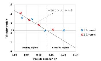
**Fig. 7.** Velocity ratio v (pebble/wall) as a function of the Froude number Fr in the 1 L (crosses) and 2 L (circles) vessels. The velocity ratio seems to be inversely proportional to the Froude number before Fr=0.13 and constant after.
