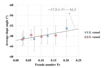
**Fig. 8.** Average slope angle of the pebble bed  $\phi$  inside the 1 L (crosses) and 2 L (circles) vessels, as a function of the Froude number Fr.
