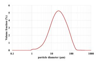
**Fig. 1.** Volume particle size distribution of the alumina GE15 powder, measured by LASER dispersion in wet mode.
