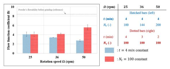
**Fig. 9.** Evolution of the flow function coefficient of ground powders according to the rotational speed of the vessel  $\Omega$  at constant grinding time t (hatched bars, left) and constant number of revolutions  $N_t$  (dotted bars, right). All the grinding tests are performed in the same filling conditions with J = 0.3 and U = 1.00.
