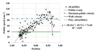
**Fig. 6.** Velocity profile of the pebbles at the surface of the pebbles bed in the 2 L vessel, rotating at 50 rpm. The velocity of a given pebble (pebble 4) is marked with the continuous dark line, the dotted curve represents the polynomial interpolation of the fall speed, the dotted straight line corresponds to the maximal velocity of the pebbles  $v_{p,max}$  and the continuous straight line corresponds to the wall linear velocity  $v_w$ .
