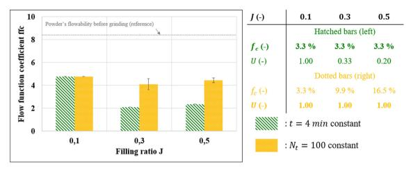
**Fig. 10.** Evolution of the flow function coefficient of ground powders according to the pebbles filling ratio J at constant powder filling ratio  $f_c$  (hatched bars, left) and constant level of powder U (dotted bars, right). All the grinding tests are performed in the same conditions with  $\Omega = 25rpm$  and t = 4min.
