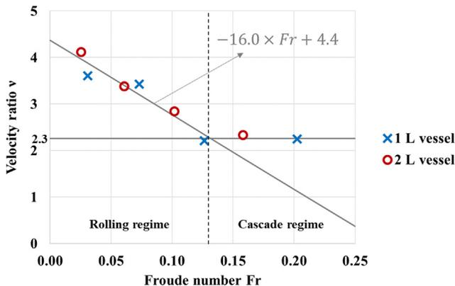
Fig. 7. Velocity ratio  $v$  (pebble/wall) as a function of the Froude number  $Fr$  in the 1 L (crosses) and 2 L (circles) vessels. The velocity ratio seems to be inversely proportional to the Froude number before  $Fr = 0.13$  and constant after.
