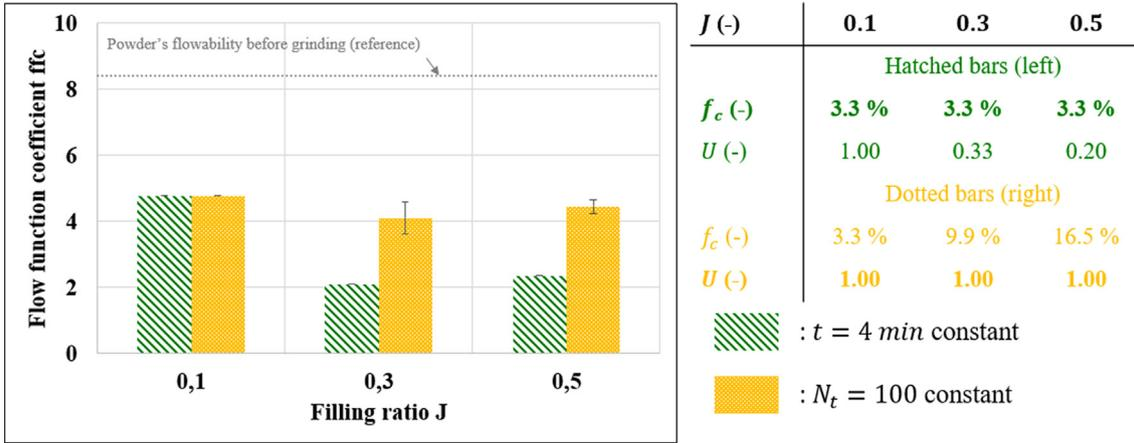
**Fig. 10.** Evolution of the flow function coefficient of ground powders according to the pebbles filling ratio  $J$  at constant powder filling ratio  $f_c$  (hatched bars, left) and constant level of powder  $U$  (dotted bars, right). All the grinding tests are performed in the same conditions with  $\Omega = 25 \text{ rpm}$  and  $t = 4 \text{ min}$ .
