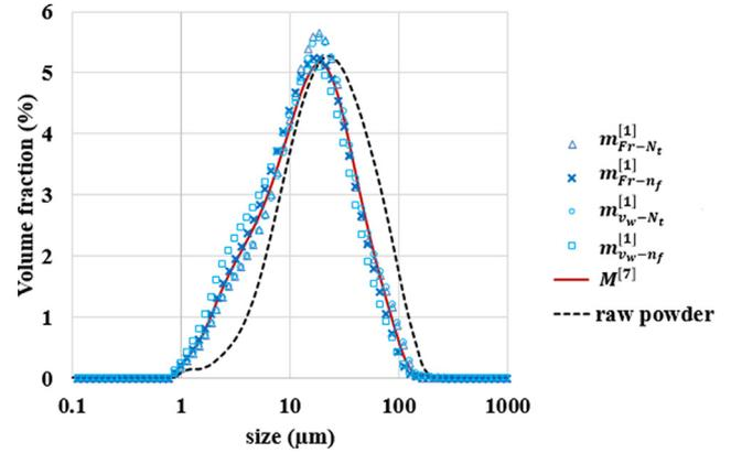
**Fig. 14.** Volume particle size distribution of the powder samples ground in the 1 L and the 7 L vessels in various conditions described in Table 7.**Table 8**Sauter mean diameters corresponding to the particle size distributions of Fig. 14 and total squared error of the particle size distribution compared to the  $M^{[7]}$  grinding test.
