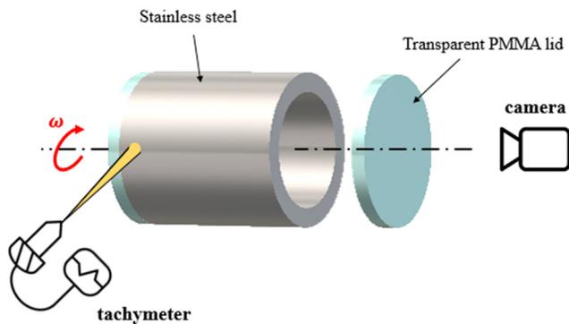
Fig. 3. Schematic representation of the ball milling setup.
