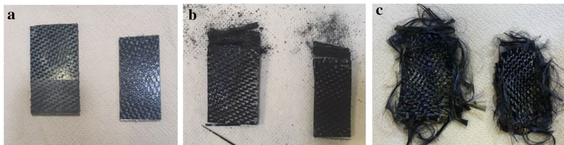
Fig. 5 a PEEK composites before recycling, b recovered solid from thermal treatment under nitrogen and c air
