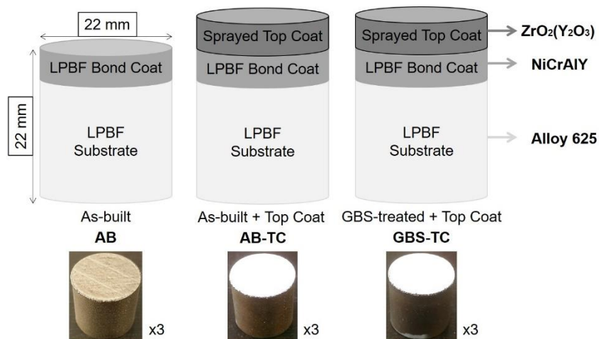
Figure 1: Schematic diagram of the specimens produced by LPBF for thermal shock testing in burner rig
