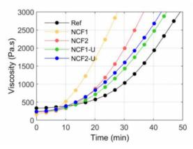
Fig. 7. Evolution of the viscosity with time at 400°C for both PEEK filaments (NCF1 and NCF2), the neat PEEK (Ref) and the NCF1 and the NCF2 filaments without sizing agents (NCF1-U and NCF2-U)
