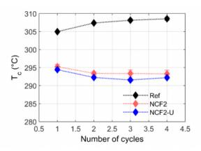
Fig. 6. The crystallization temperature  $T_c$  (°C) as a function of number of cycles for the NCF2 and the NCF2-U semi-finished products, with and without sizing agents respectively and the neat PEEK (Ref)
