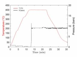
Fig. 2. Monitoring of temperature and applied pressure during a thermo-compression cycle of 400°C during 10 min under 9 bars
