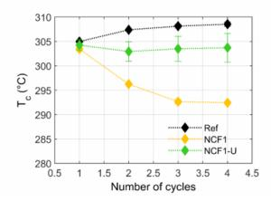
Fig. 5. The crystallization temperature  $T_c$  (°C) as a function of number of cycles for the NCF1 and the NCF1-U semi-finished products, with and without sizing agents respectively and the neat PEEK (Ref)
