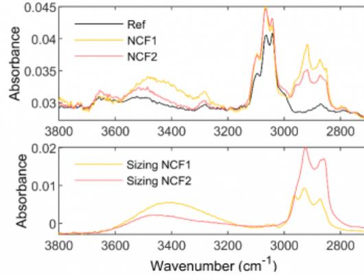
Fig. 4. FTIR spectra: on the top the different semi-finished products (NCF1 and NCF2) and the neat PEEK (Ref), on the bottom the sizing agents of NCF1 and NCF2
