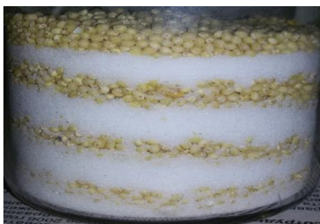
Fig. 4. The experimental set-up (a) and fragment of components distribution (b) at multilayer loading
