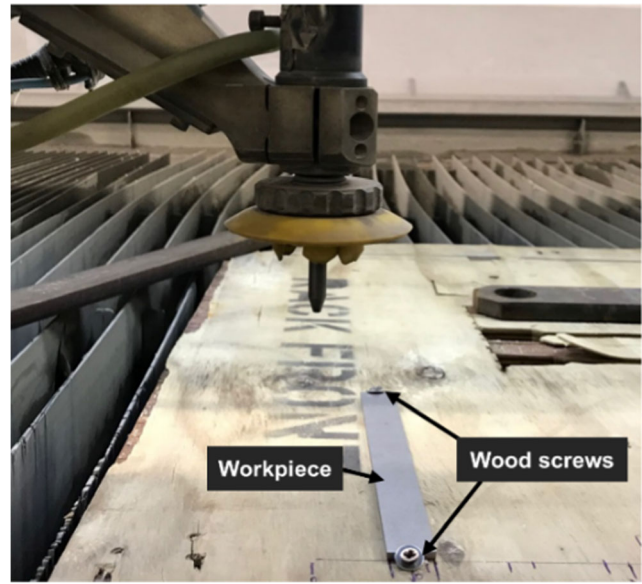
Fig. 1 Experimental setup for AWJ milling
