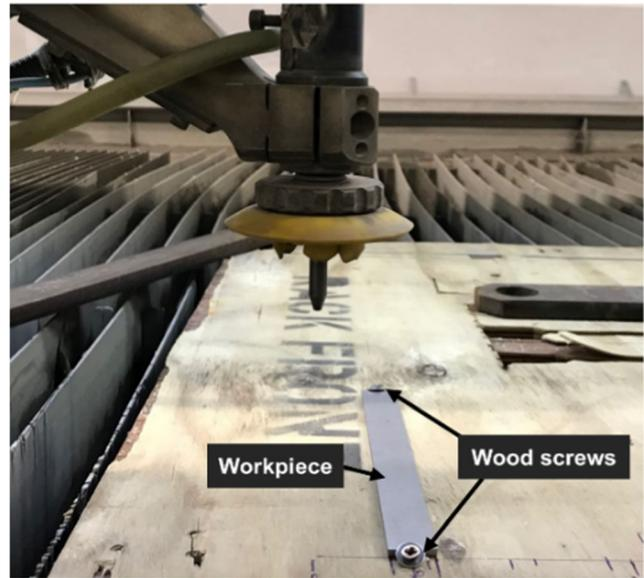
Fig. 1 Experimental setup for AWJ milling
