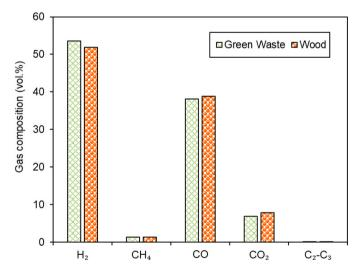
**Fig. 9.** Composition of syngas from green waste and wood after reforming at 1300  $^{\circ}$ C and a gas residence time of 5 s.
