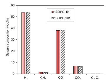
Fig. 7. Syngas composition from green waste after reforming at 1300  $^\circ\text{C}$ , with the gas residence time of 5 s and 10 s.
