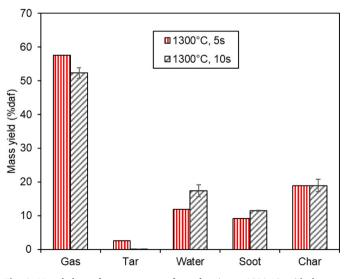
Fig. 6. Mass balance for green waste after reforming at 1300  $^\circ\text{C}$ , with the gas residence time of 5 s and 10 s.
