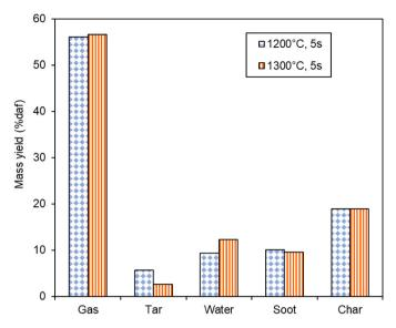
Fig. 4. Mass balance for green waste after reforming at 1200  $^\circ C$  and 1300  $^\circ C$ , with a gas residence time of 5 s.
