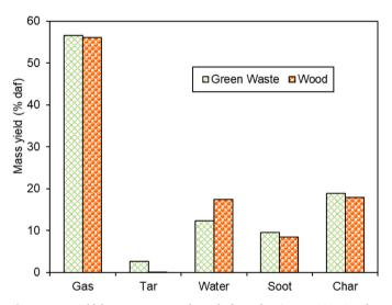
Fig. 8. Mass yield for green waste and wood after reforming at 1300  $^\circ$ C and a gas residence time of 5 s.
