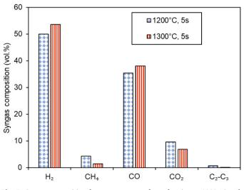
Fig. 5. Syngas composition from green waste after reforming at 1200  $^\circ C$  and 1300  $^\circ C$ , with a gas residence time of 5 s.
