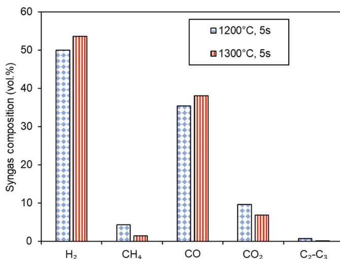
Fig. 5. Syngas composition from green waste after reforming at 1200 °C and 1300 °C, with a gas residence time of 5 s.
