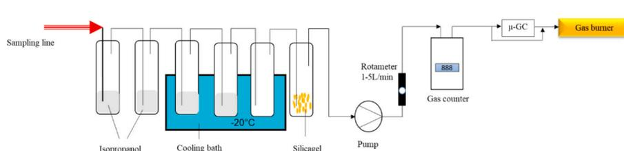
**Fig. 2.** Gas and bio-oil sampling system.
