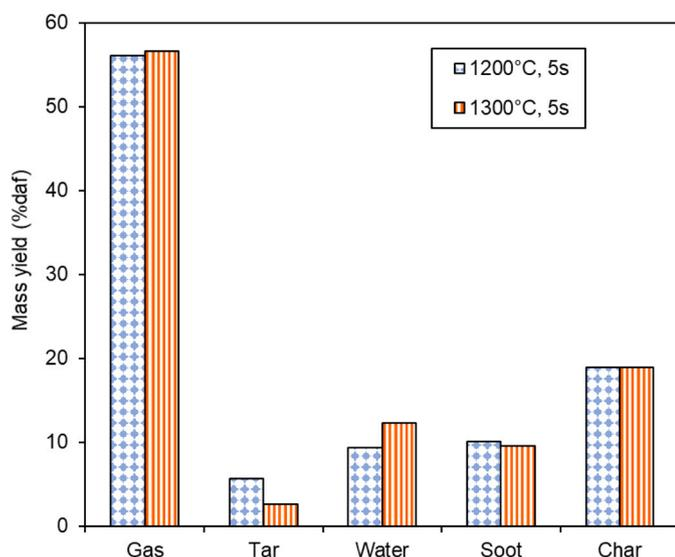
Fig. 4. Mass balance for green waste after reforming at 1200 °C and 1300 °C, with a gas residence time of 5 s.
