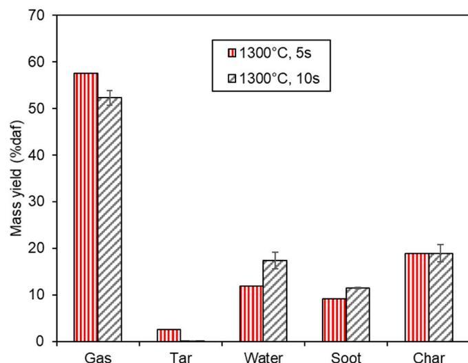
Fig. 6. Mass balance for green waste after reforming at 1300 °C, with the gas residence time of 5 s and 10 s.
