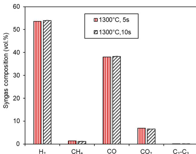
Fig. 7. Syngas composition from green waste after reforming at 1300 °C, with the gas residence time of 5 s and 10 s.
