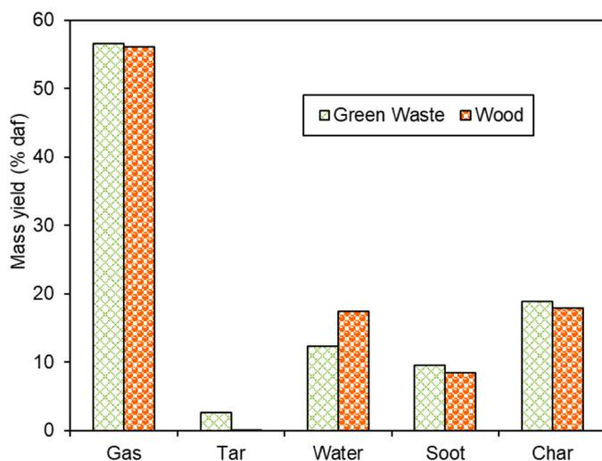
**Fig. 8.** Mass yield for green waste and wood after reforming at 1300 °C and a gas residence time of 5 s.
