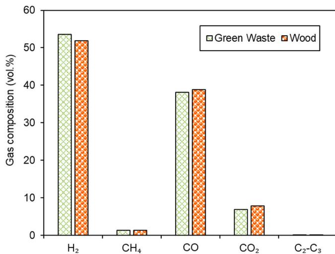
**Fig. 9.** Composition of syngas from green waste and wood after reforming at 1300 °C and a gas residence time of 5 s.
