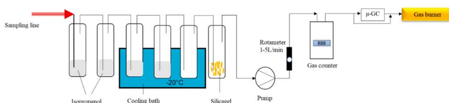
**Fig. 2.** Gas and bio-oil sampling system.
