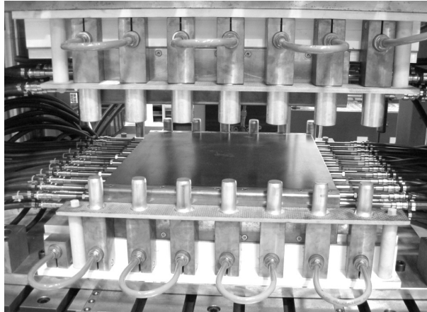
Figure 4 – Cage System ® induction heated mould
