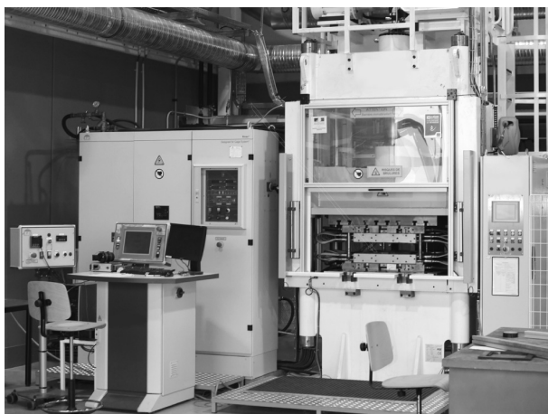
Figure 8 – Thermo-compression pilot plant with induction-heated mould
