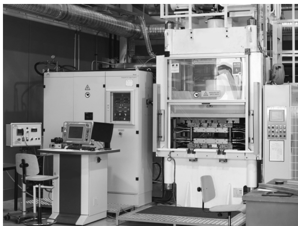
Figure 8 – Thermo-compression pilot plant with induction-heated mould
