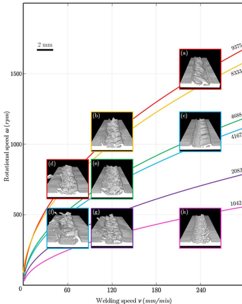
Fig. 6. 3D reconstructed images corresponding to the Ti-6Al-4V distribution inside Al2024 according to welding and rotational speeds. Isolines correspond to the values of  $\omega^2/\nu$  (given in  $\text{rad}^2 \text{mm}^{-1} \text{s}^{-1}$ ) of the welds.
