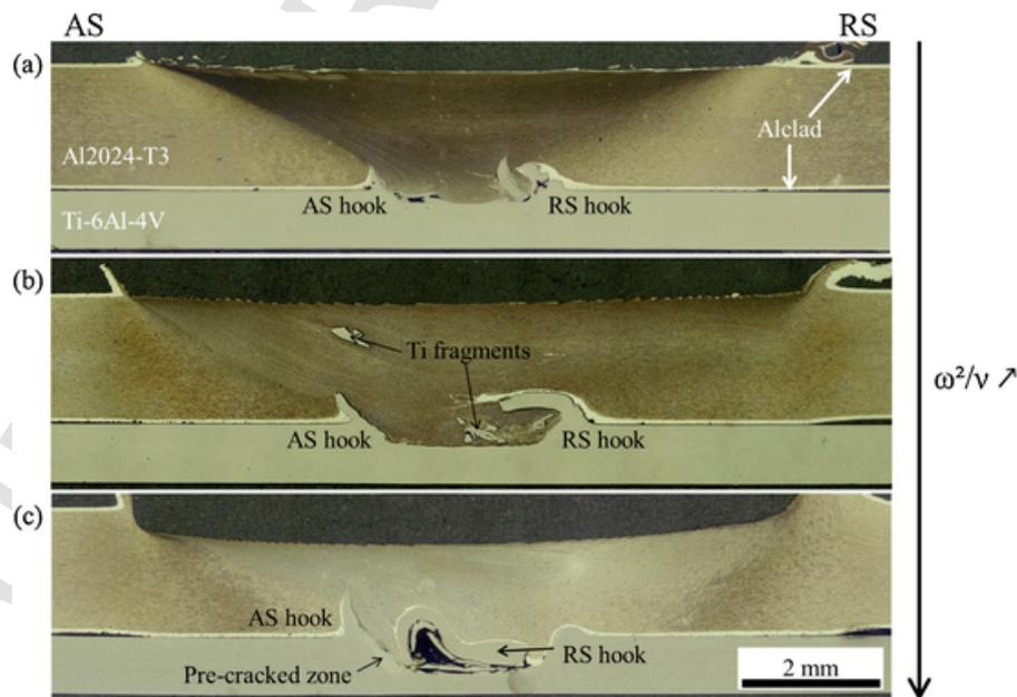
Fig. 18. Optical microscope images of the welds cross sections: (a) weld 3; (b) weld 1 and (c) weld 11 sorted in ascending order of  $\omega^2/\nu$  increasing. Note that weld 11 was produced with an improper welding condition (leading the tool plunge through the Al2024 top plate and the perforation of the Ti-6Al-4V bottom plate).
