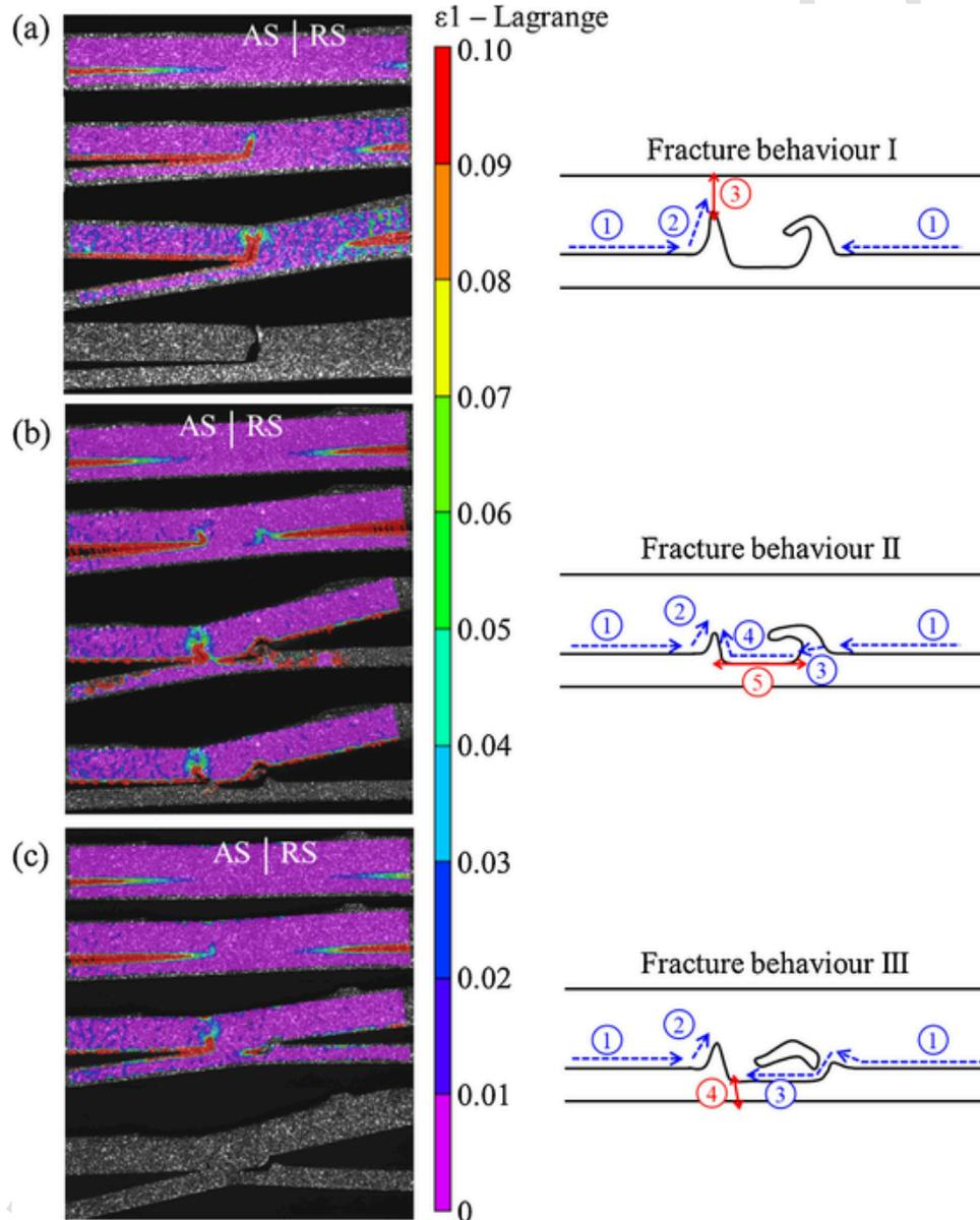
Fig. 13. Evolution of the strain fields, along cross sections, evaluated by digital image correlation and schematics on the three fracture behaviours: (a) FB I; (b) FB II; (c) FB III. Note that  $\epsilon_1$  represents the major principle strain.
