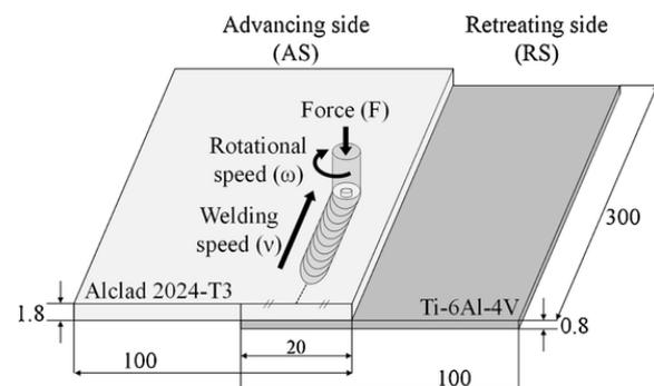
**Fig. 1.** Schematic illustration of a FSW Al2024-T3/Ti-6Al-4V lap joint (dimensions in mm).
