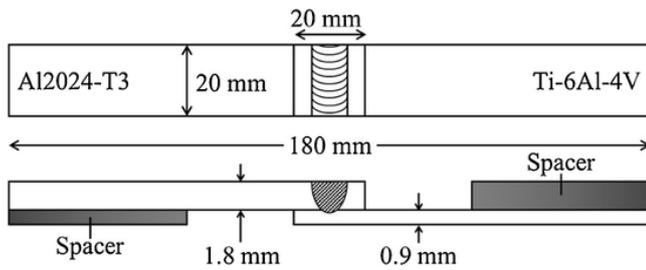
Fig. 3. Schematic illustration of lap shear specimen.
