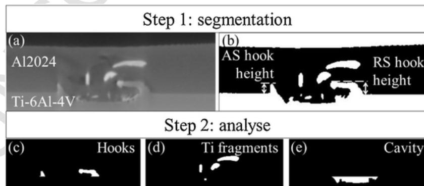
**Fig. 2.** (a) CT-scan images used for post-processing procedures; (b) segmentation for binary images and analyse of (c) the Ti-6Al-4V hooks; (d) the Ti fragments penetrated inside the aluminium alloy plate and (e) the cavity formed by the pin penetration in the titanium alloy plate.
