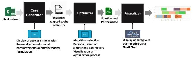
Fig. 1 Architecture of the research prototype BLPAD.Core
