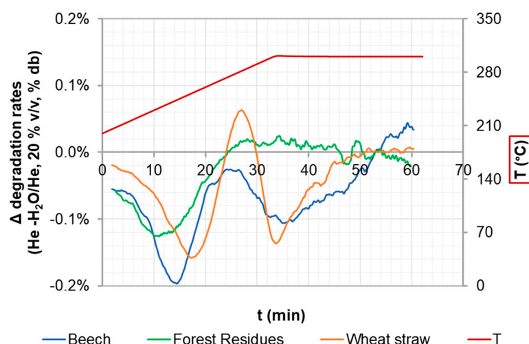
Figure 7. Instantaneous difference in degradation rate versus time and temperature from TGA results of the torrefaction of beech, forest residues and wheat straw under dry (He, 100% v/v ) and moist (H 2 O/He, 20% v/v ) atmospheres.
